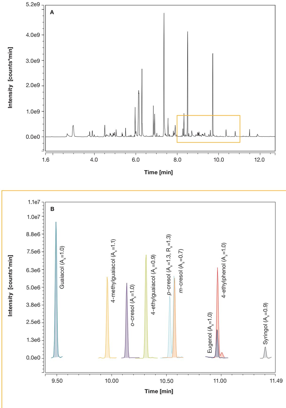
Figure 1. TIC (full scan:  $m/z$  50–500, A-upper trace) and SRM acquisition (B-bottom trace) for a wine sample spiked at 5  $\mu\text{g/L}$ . Chromatographic separation was achieved for all the investigated compounds with the exception of eugenol and 4-ethylphenol ( $\text{RT}=10.92$  min) that can be easily separated based on their characteristic ions.  $A_s$  values and  $R_s$  for the critical pair  $p,m$ -cresol are annotated.
