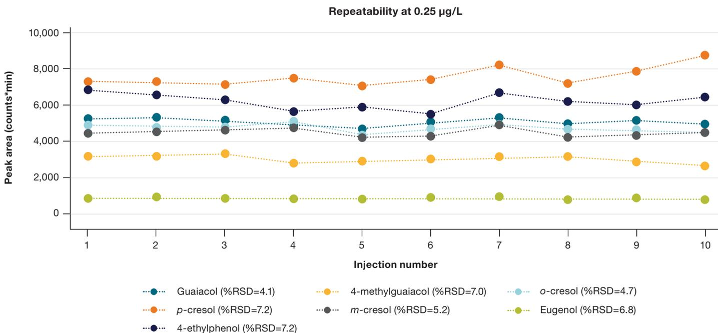
Figure 4. Precision of measurement as peak area %RSDs obtained for n=10 consecutive extractions at 0.25  $\mu\text{g/L}$  were <10%.
