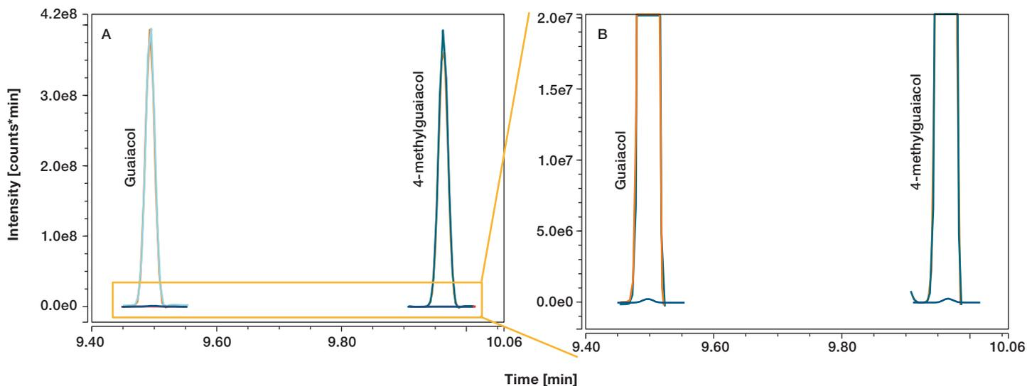
Figure 3. Example of carryover (blue trace) assessed running a fiber blank after extraction of wine samples (n=2) spiked at 500  $\mu\text{g/L}$ , full scale (A), zoomed scale (B). Calculated carryover for both guaiacol and 4-methylguaiacol was <0.10%.
