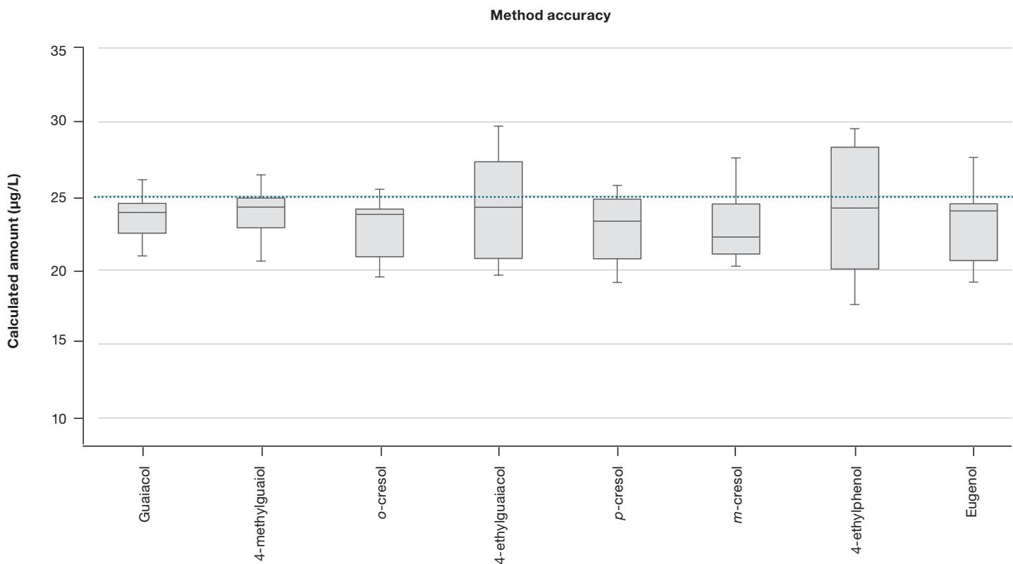
**Figure 5. Robust performance as demonstrated by the analysis of QC standards spiked at 25 µg/L and injected every six samples.** The calculated amounts were within 20% of the expected concentration for all compounds.
