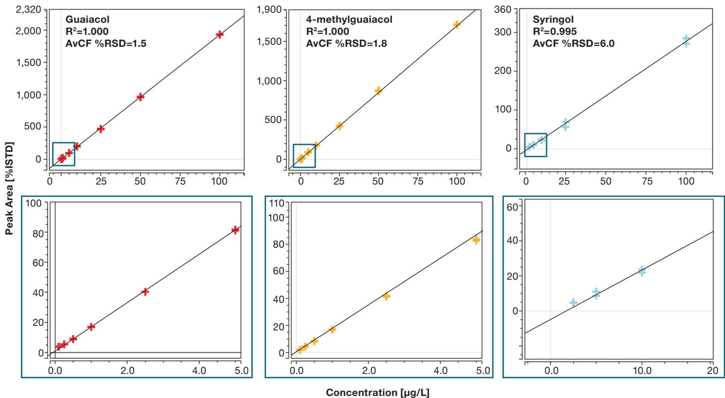
Figure 2. Examples of calibration curves for guaiacol, 4-methylguaiacol, and syringol. Each calibration level was injected in duplicate. Coefficient of determination ( $R^2$ ) and AvCF %RSD are annotated.
