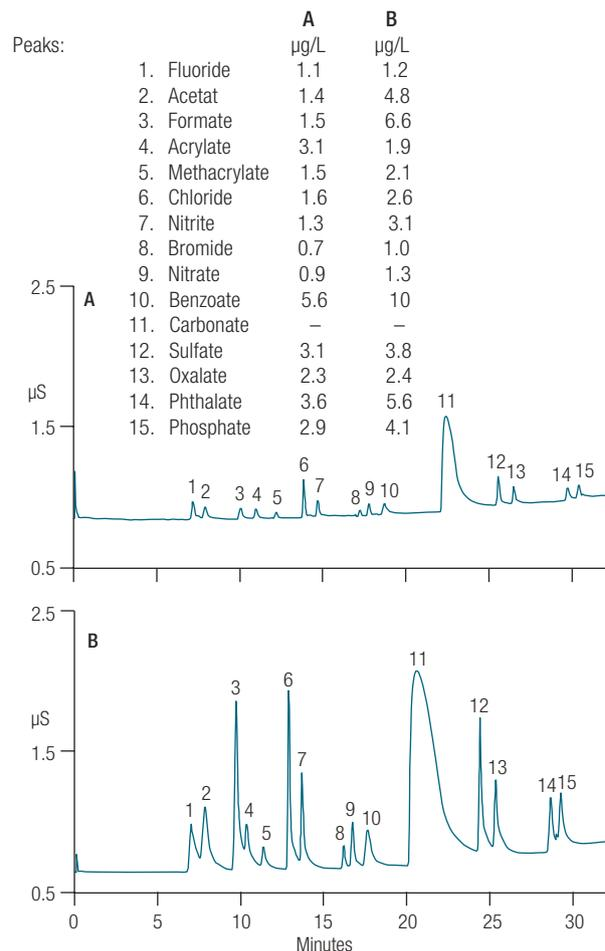
Figure 3. Trace anion standard analyses.
