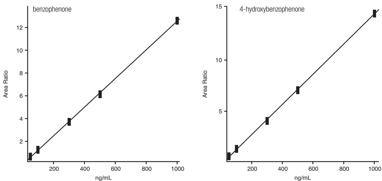
Figure 2: Calibration curve for benzophenone and 4-hydroxybenzophenone
