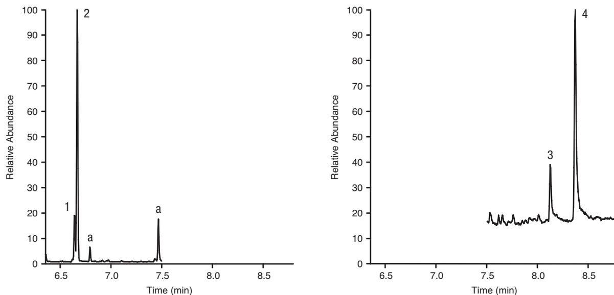
Figure 3: SIM chromatogram for benzophenone and 4-hydroxybenzophenone spiked at 0.6 mg/kg in breakfast cereal
