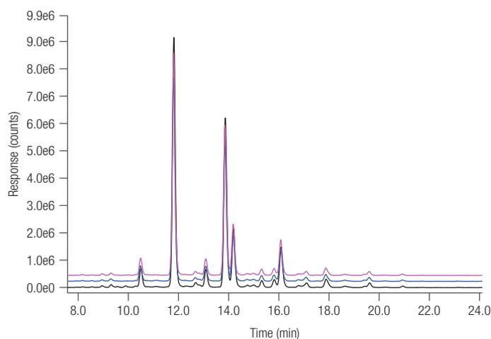
**Figure 1. Overlay of replicate analysis of *N*-glycans released from NISTmAb following separation on an Accucore Amide-150 HILIC column and a Vanquish Flex UHPLC.**
