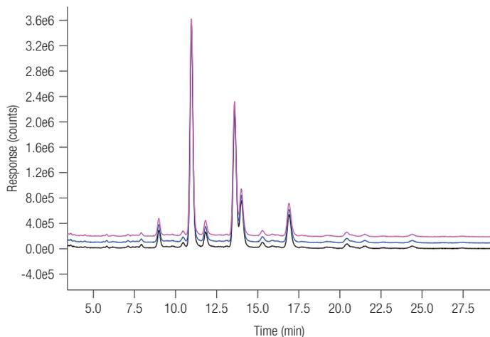
**Figure 2. Separation of N-glycans released from NISTmAb following separation on a GlycanPac AXH-1 column and a Vanquish Flex UHPLC.**
