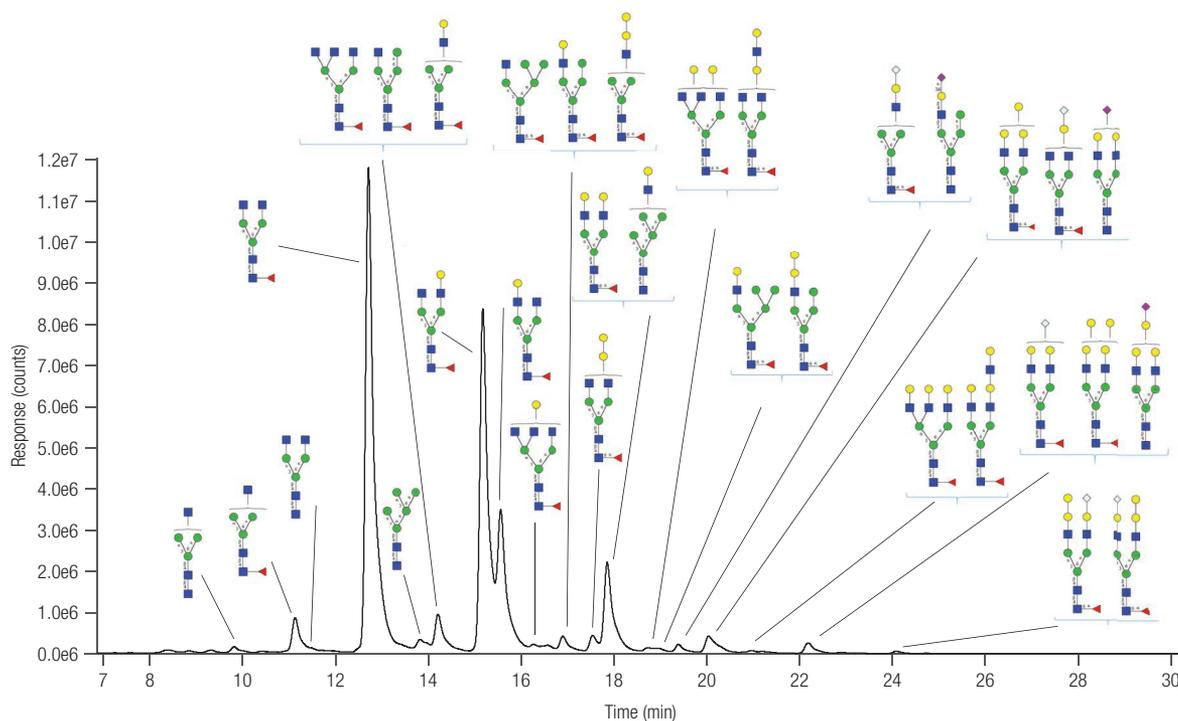
**Figure 3. Identification of N-glycans released from NISTmAb following separation on an Accucore Amide-150 HILIC column and a Vanquish Flex UHPLC coupled to a Q Exactive Plus hybrid quadrupole-Orbitrap mass spectrometer with the Biopharma option. Glycan structures are annotated according to the Consortium for Functional Glycomics (CFG) system.<sup>4</sup>**
