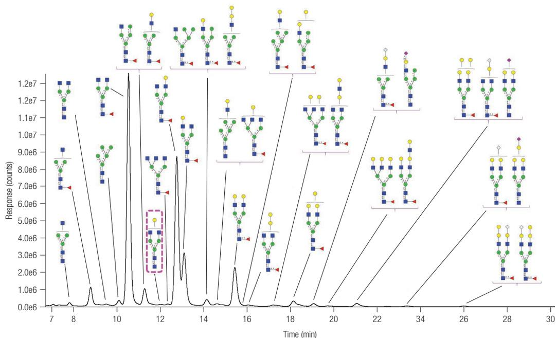
Figure 4. Identification of N-glycans released from NISTmAb following separation on a GlycanPac AXH-1 column and a Vanquish Flex UHPLC coupled to a Q Exactive Plus hybrid quadrupole-Orbitrap mass spectrometer with the Biopharma option. Glycan structures are annotated according to the Consortium for Functional Glycomics (CFG) system.<sup>4</sup> The glycan structure A2G1 is highlighted in pink.
