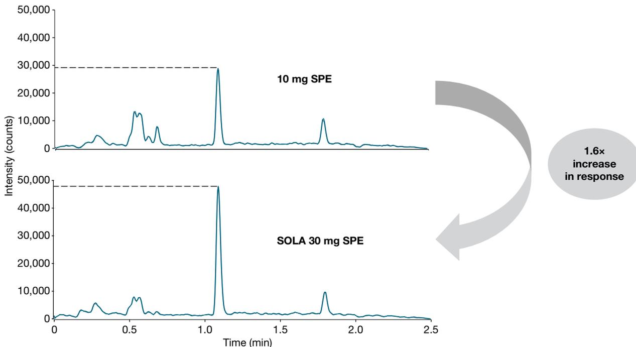
**Figure 7. The high loading capacity of SOLA HRP 30 mg also improves signal response when compared to smaller bed weights.** The chromatograms show an improved signal response of OH-Vit D<sub>3</sub> for SOLA HRP 30 mg after human plasma (1 mL) was spiked at MQC level and loaded onto each bed weight.
