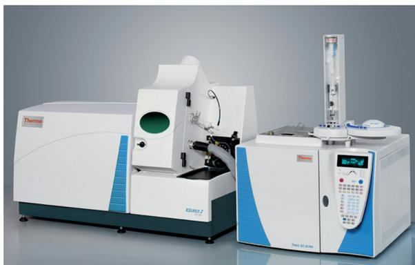
Figure 1: Thermo Scientific TRACE GC Ultra coupled to the XSERIES 2.
