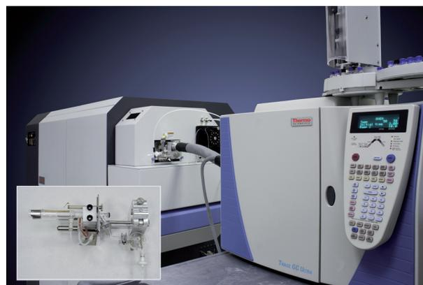
Figure 2: TRACE GC Ultra™ coupled to the ELEMENT 2.
