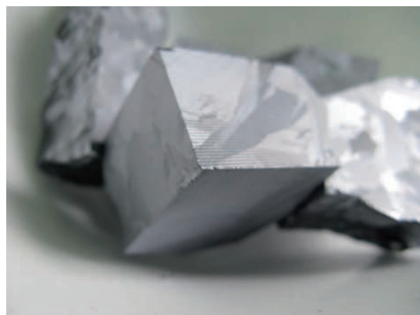
Figure 3. Bricks of multicrystalline silicon base material for the production of solar cells.
