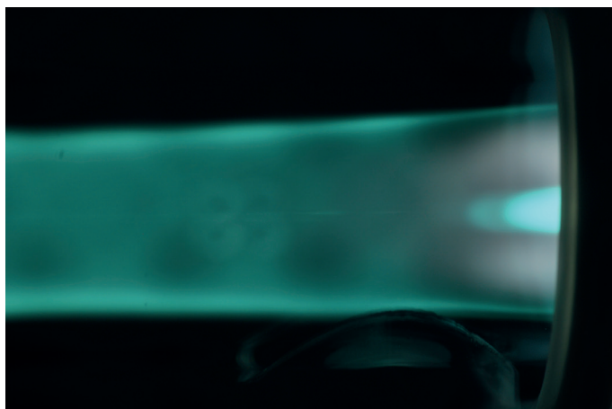
Figure 1. Aspirating 1-pentanol into the plasma after the nebulizer gas flow has been adjusted.
