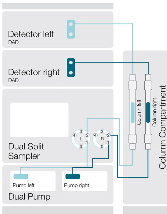
Figure 1. Fluidic setup of Vanquish Flex Duo UHPLC system.
