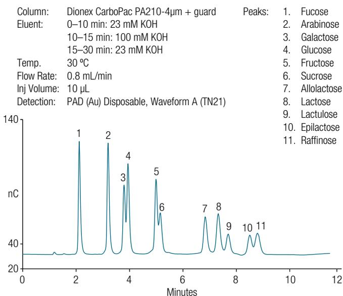
Figure 1. Chromatogram of a 5 ppm sugar standard mix
