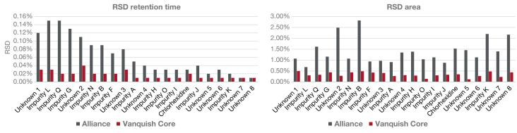
Figure 3. Relative standard deviations (RSD) of retention times and peak areas over seven injections obtained by the Alliance and Vanquish Core HPLC systems
