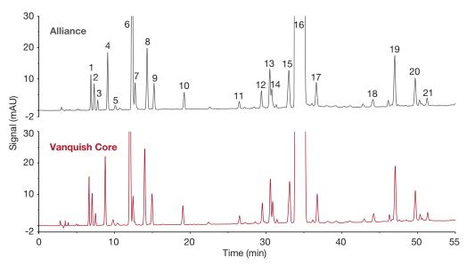
Figure 1. Transfer from Alliance system to Vanquish Core HPLC system according to the EP monograph for chlorhexidine gluconate; peak assignment according to impurity designation in EP monograph and standard leaflet<sup>5,9</sup>
