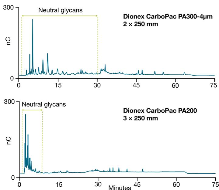
**Figure 5. Comparison of chromatographic traces of porcine gastric mucin type III O-glycans on the Dionex CarboPac PA200 (bottom) and Dionex CarboPac PA300-4 $\mu$ m (top) columns. The approximate window during which neutral glycans elute is highlighted in the arrowed region.**
