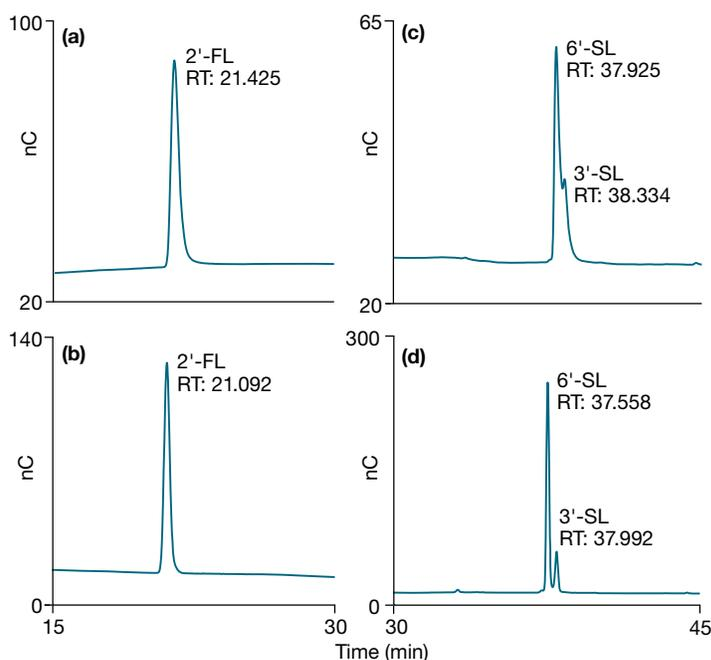
Figure 10. PAD chromatograms of three milk oligosaccharides: (a) and (c) with an exhausted a Dionex ERD 500, (b) and (d) without a Dionex ERD 500
