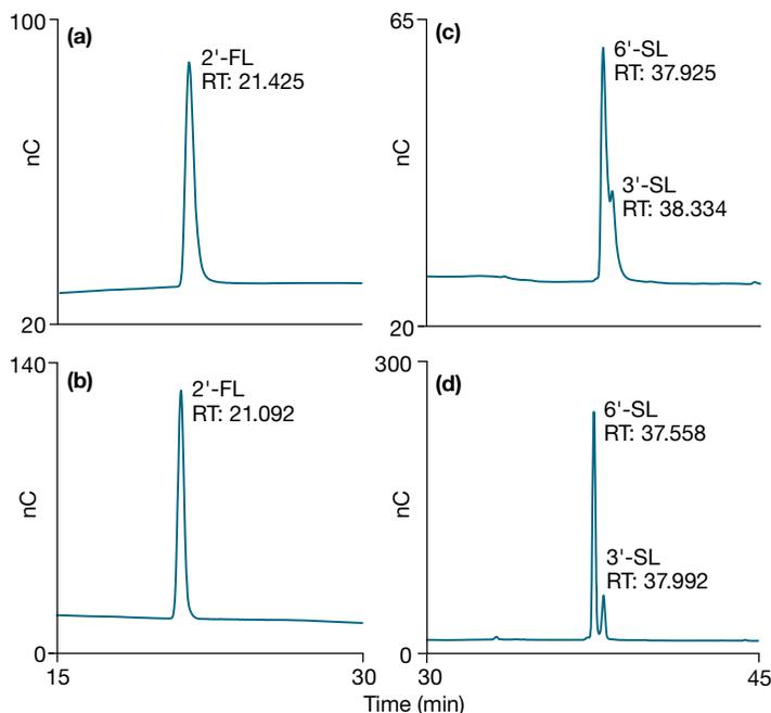
Figure 10. PAD chromatograms of three milk oligosaccharides: (a) and (c) with an exhausted a Dionex ERD 500, (b) and (d) without a Dionex ERD 500
