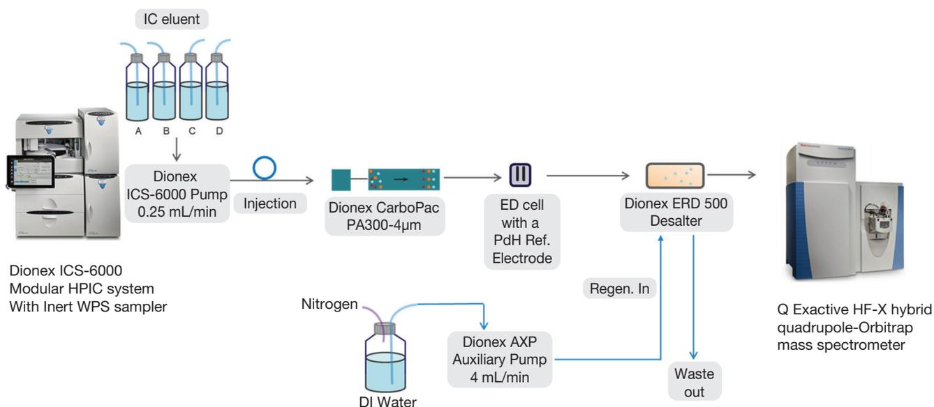
Figure 2. The system configuration of HPAE-PAD with a PdH reference electrode hyphenated to Q Exactive Orbitrap Mass Spectrometer
