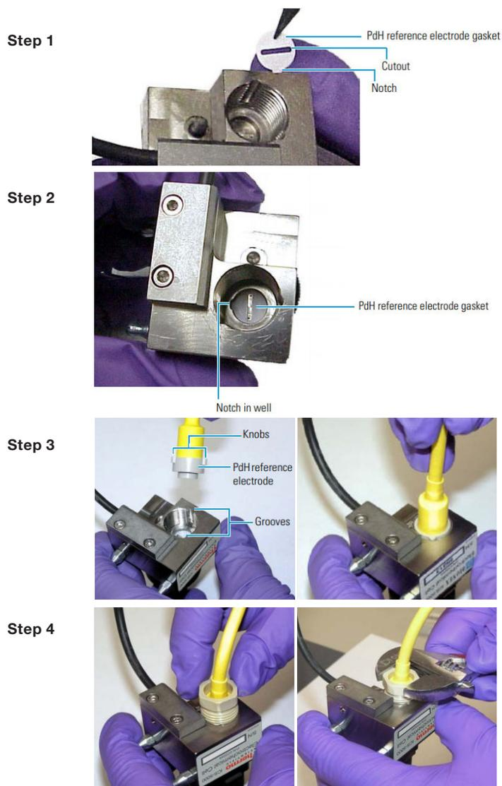
Figure 3. Overview of the installation of a palladium hydrogen (PdH) reference electrode
