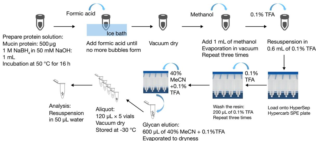
Figure 1. Sample preparation and purification workflow for O-glycans
