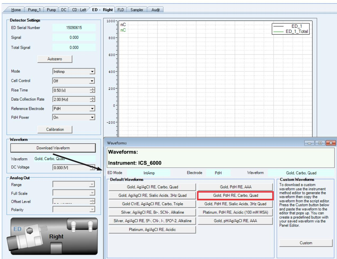
Figure 4. The choice of a correct waveform for carbohydrate analysis using a PdH reference electrode
