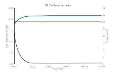
Figure 1: Sensor reads of the Cytomat 2 C450-LiN ToS incubation chamber. A graph showing gas concentration (vol%) and temperature (°C) against time (sec). The red line indicates temperature, the blue line shows the percentage of  $O_2$  and the black line represents the percentage of  $O_2$  in the chamber. Air purging starts at t=0 sec.
