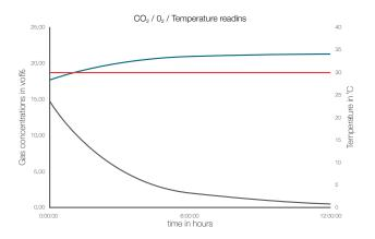
Figure 2: Sensor reads of chamber conditions – a close up view. A graph showing gas concentration (vol%) and temperature (°C) against time (sec). The red line indicates the temperature, the blue line shows the percentage of O2 and the black line represents the percentage of CO2 in the chamber. Air purging starts at t=0 sec.
