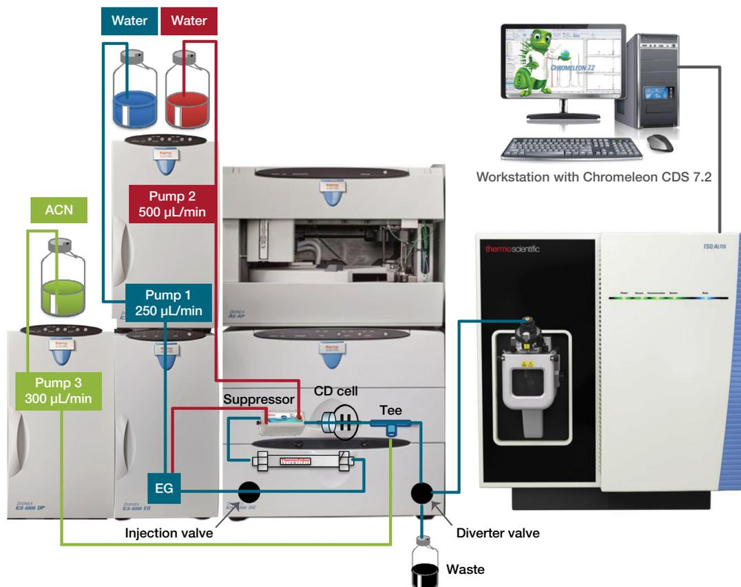
Figure 1. Schematic flow path for the IC-MS/MS setup
