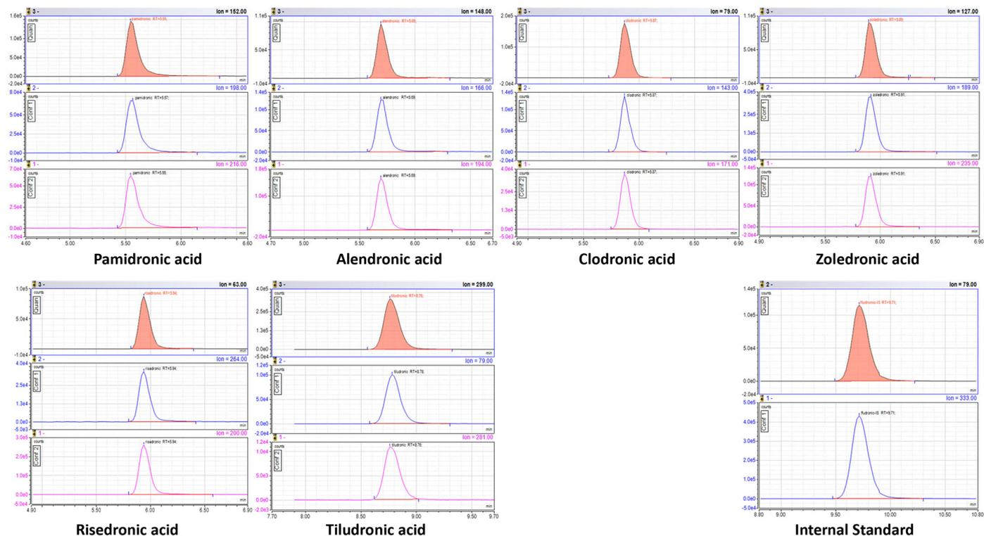
Figure 3. SRM chromatographic representation of seven bisphosphonates monitored with the TSQ Altis MS (standard solution at 1  $\mu\text{g}/\mu\text{L}$ )
