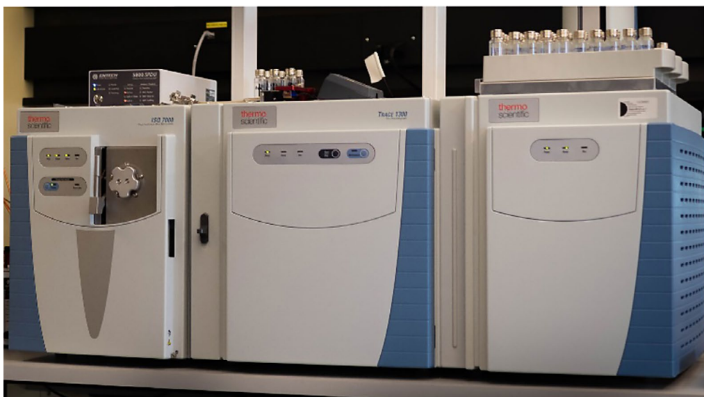
Figure 2. TriPlus 500 Headspace Autosampler, TRACE 1300 Gas Chromatograph, and ISQ 7000 Single Quadrupole GC-MS
