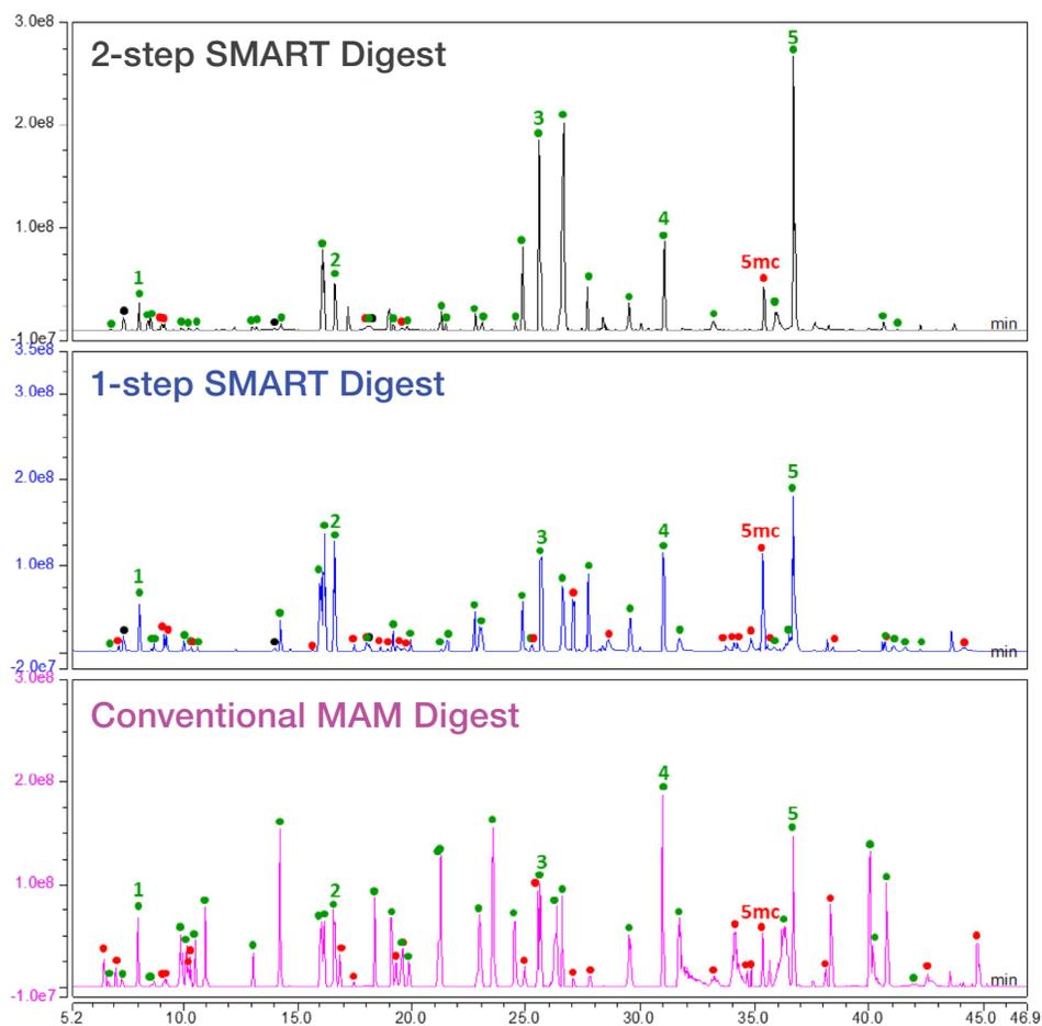
Figure 1. Base peak chromatograms (BPCs) of NISTmAb digested with the two-step SMART digest method, the original one-step SMART digest method, and the conventional MAM digest method. Missed cleavages are indicated in red (5 mc highlighted to show variation in intensity of a constant missed cleavage across all methods).
