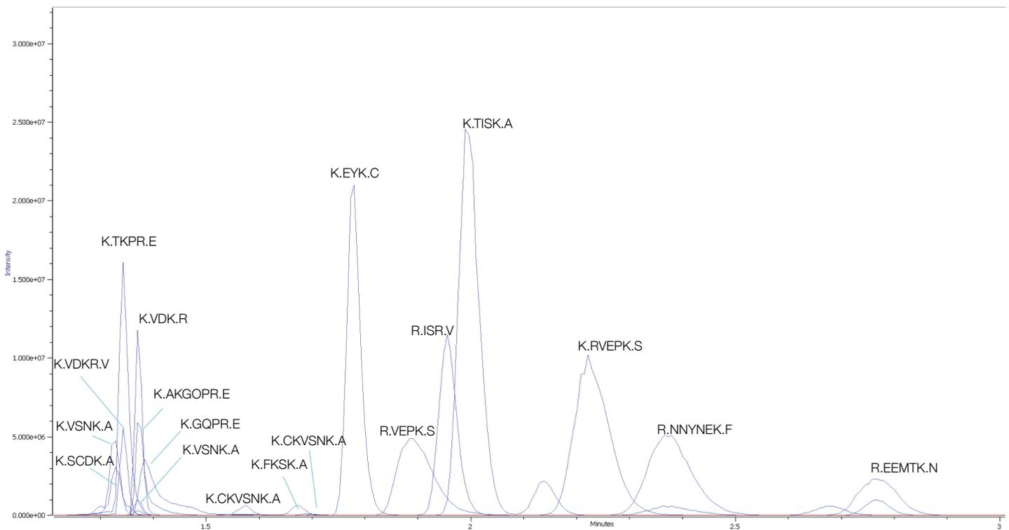
Figure 3. Identified early eluting peptides from 1 to 3 min on C4 column, confirming the MS switching time is required to be optimized to include peptides eluted earlier than the original 3 min switching valve time.
