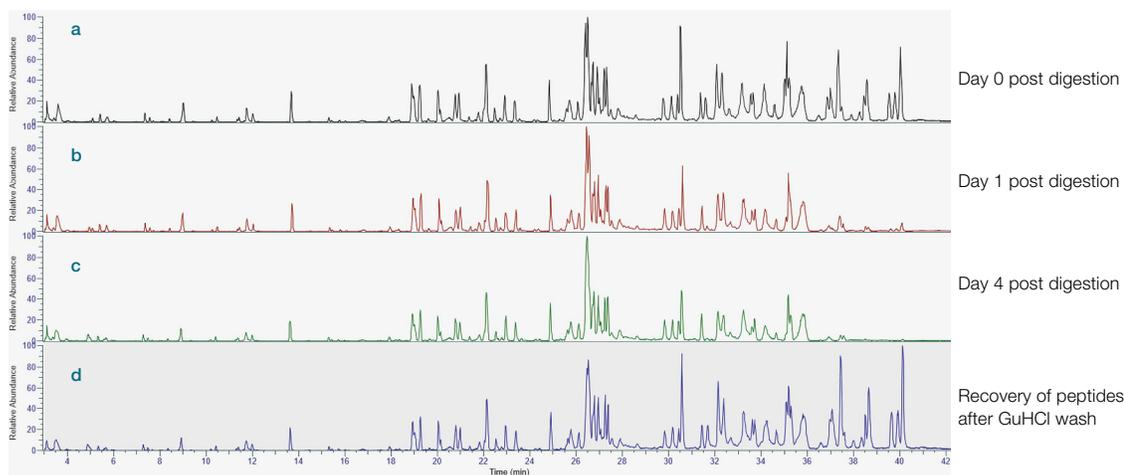
**Figure 6. Time course experiment showing the loss of hydrophobic peptide over time (traces a,b,c) and recovery of hydrophobic peptides by addition of 4 M GuHCl (trace d).**
