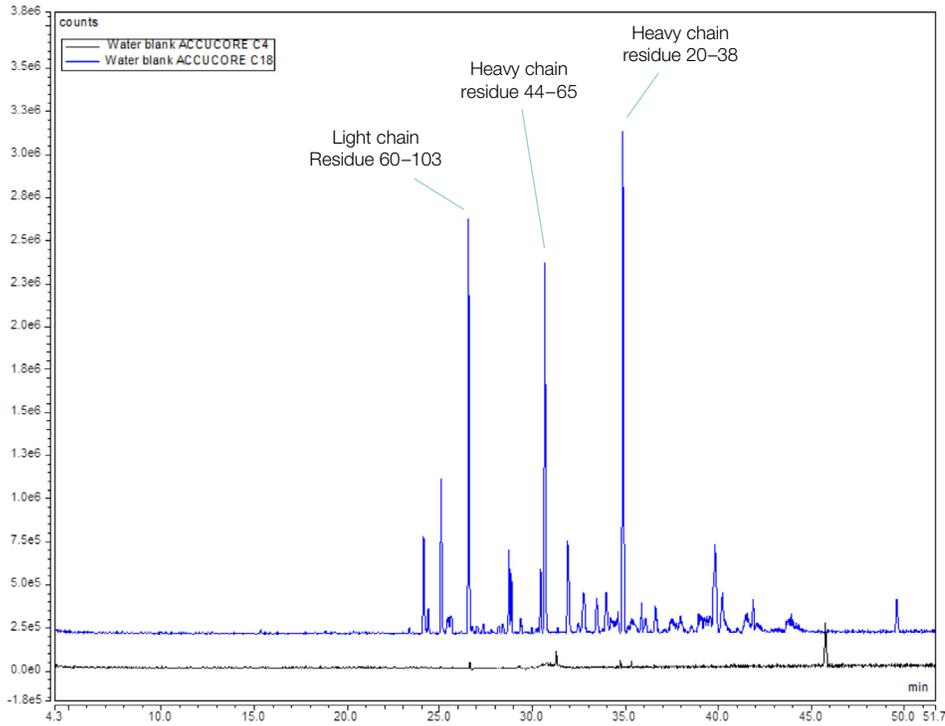
Figure 4. Base peak chromatograms obtained from runs with blank injections using the C4 (black) and C18 (blue) columns, each performed right after a series of injections of Project 3 mAb 2 digest sample. Identities of the three main peaks in the blue chromatogram were assigned via MS/MS.
