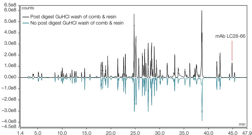
**Figure 7. Comparison of base peak chromatograms obtained from procedures with (black trace) and without (teal trace) additional 8 M GuHCl wash steps. The strongest effect upon including the GuHCl wash step is observed for the late-eluting peptide mAb LC28-66 showing a significantly increased signal intensity. GuHCl wash step (top, black trace) versus much lower intensity of LC25-66 without the GuHCl wash (lower, teal trace).**
