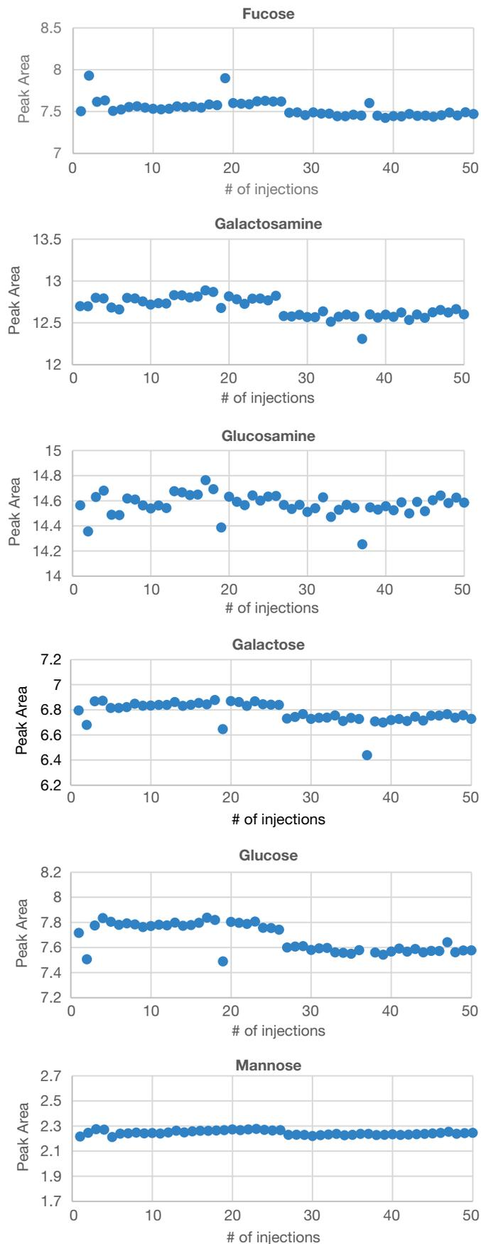
Figure 14. Electrochemical response stability of six monosaccharides over 50 consecutive injections (using a PdH RE)
