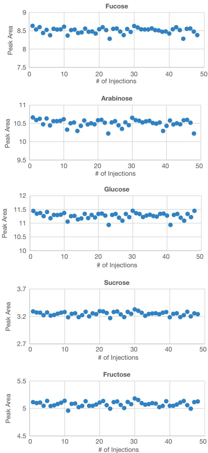
Figure 13. Electrochemical response stability of five sugars over 50 consecutive injections (using a PdH RE)
