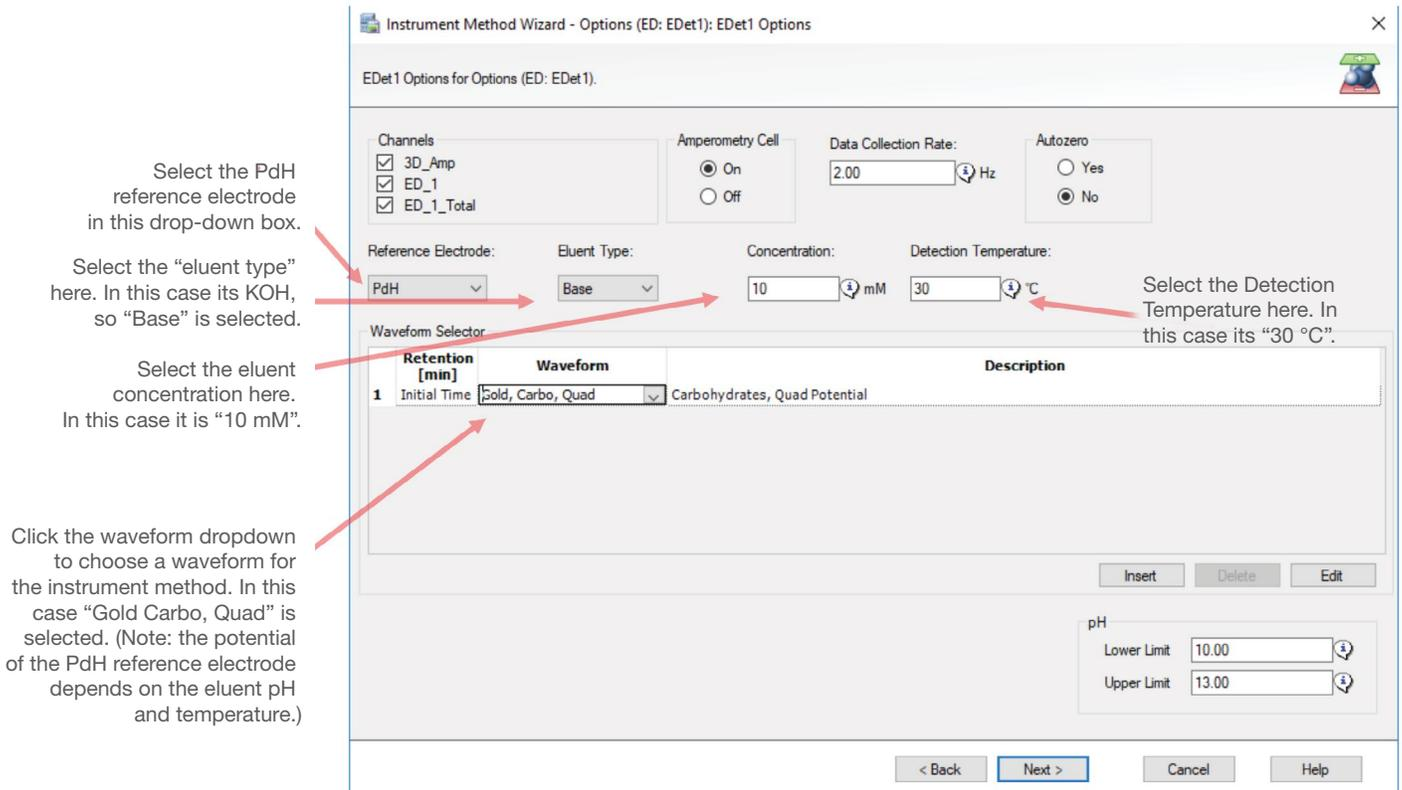
Figure 3. Creating an instrument method for using a PdH reference electrode
