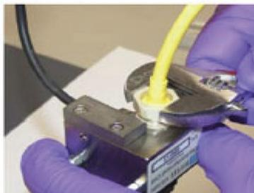
Figure 1. Stepwise installation of a PdH reference electrode
