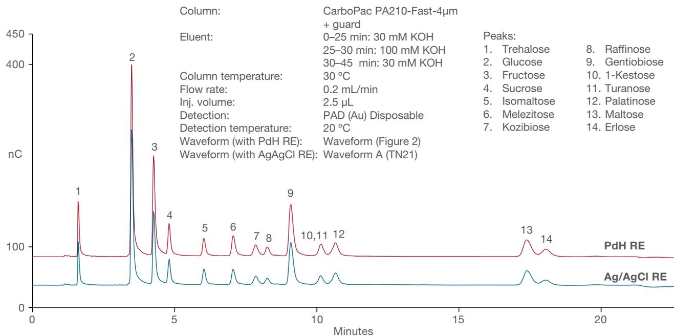
Figure 6. Comparison of the 14 honey sugar mixed standard run using PdH and Ag/AgCl reference electrodes
