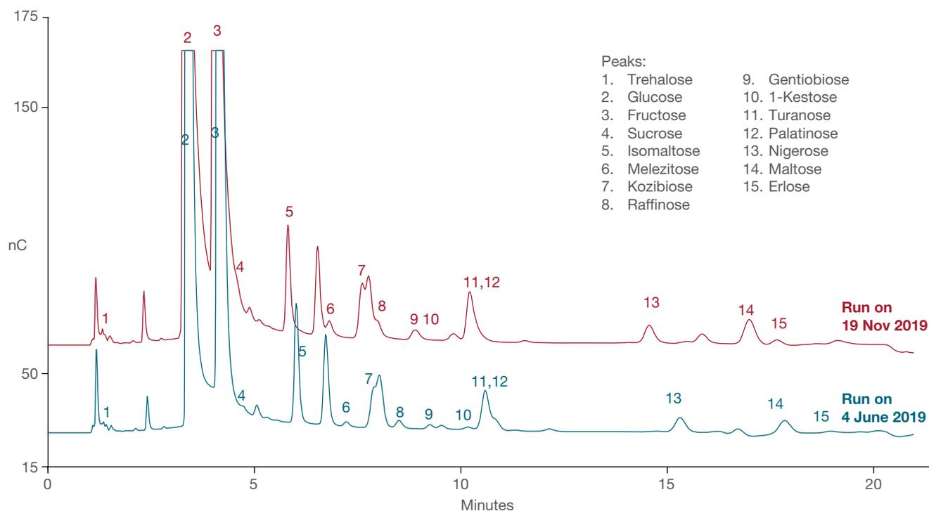
**Figure 15. Chromatogram of honey sample 1, run using the same PdH reference electrode 6 months apart**
