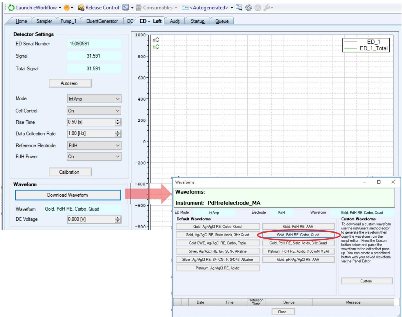
Figure 2. Picking a waveform from the ED panel
