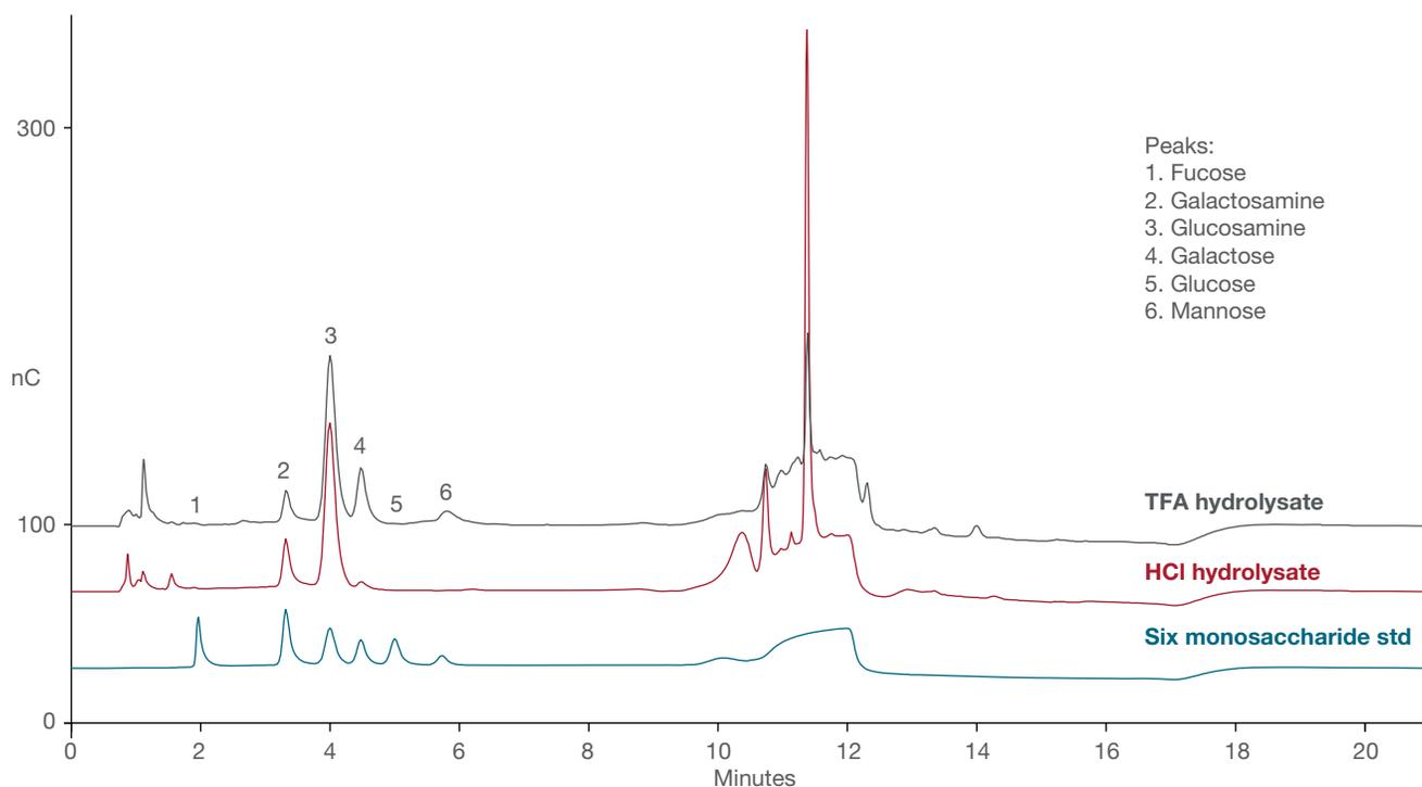
Figure 12. Chromatogram of bovine fetuin TFA and HCl hydrolysates using PdH reference electrode
