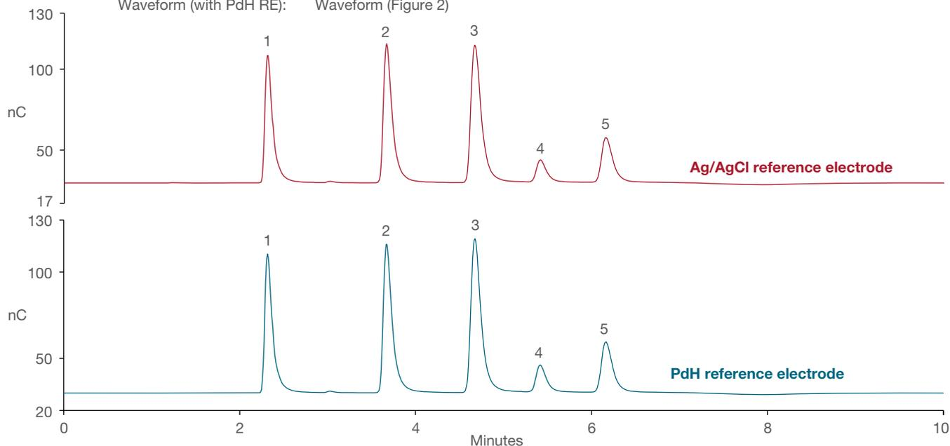
Figure 5. Chromatograms of the column's QAR standard using PdH and Ag/AgCl reference electrodes
