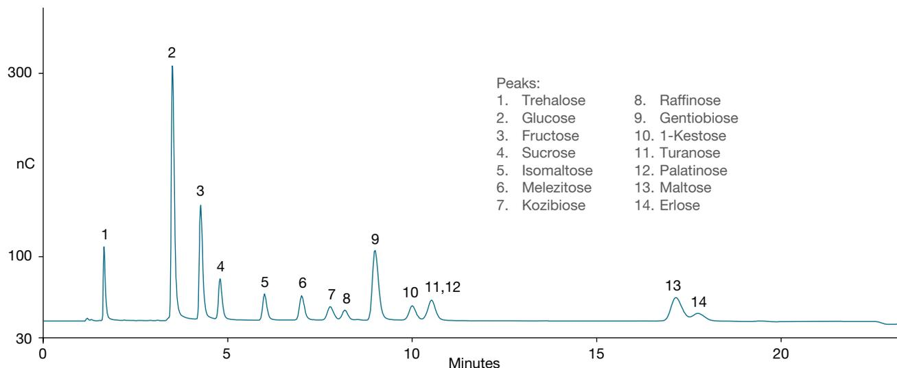
Figure 7. Chromatograms of a 14 honey sugar mixed standard run at 29 mM KOH using a PdH reference electrode
