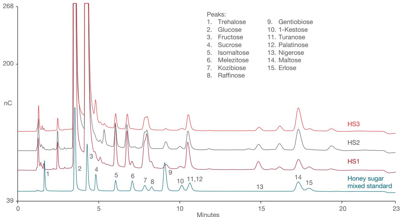
Figure 9. Chromatograms of three honey samples run @ 30 °C using a PdH reference electrode
