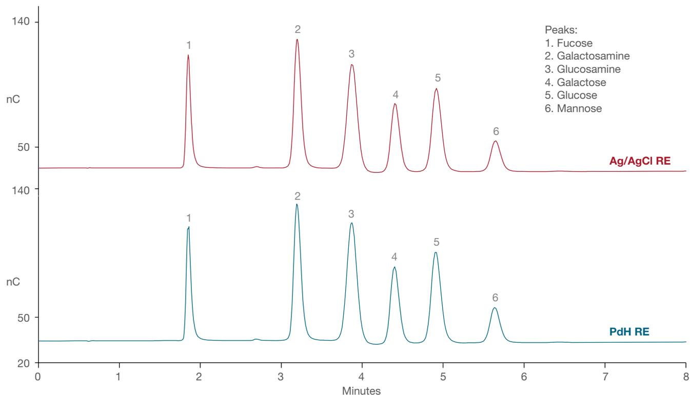
Figure 10. Chromatogram of the column's QAR standard using Ag/AgCl and PdH reference electrodes
