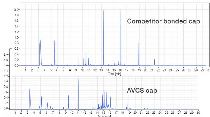
Chromatograms show the background peaks for two different cap technologies (shown in the same scale). Less background peaks result from the AVCS cap compared to the competitor bonded cap.
