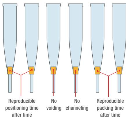
This innovative design enables high levels of reproducibility when dealing with highly complex biological samples, not only from cartridge-to-cartridge or well-to-well but also batch-to-batch when compared to conventional SPE products.
