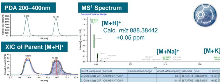
**Figure 3. Correlation of the main UV peaks with the XIC of 5'-DMT-2'-Ome-A(bz)-CEP in Compound Discoverer, with the MS1 spectrum at apex showing the isotopic peak pattern matching the expected elemental composition within tolerances (green bars).**
