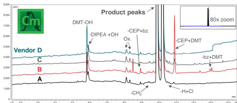
**Figure 2. Overlay of the total UV spectra for 5'-DMT-2'-Ome-A(bz)-CEP from all four vendors, zoomed in to show the different trace impurity peaks, using Chromeleon CDS.**
