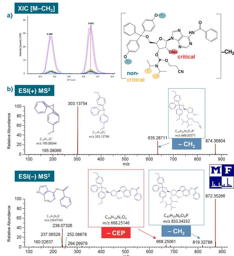
**Figure 6. a) Impurity at 9.37/9.65 min with possible demethylation sites highlighted. b) Fragmentation spectra of [M+H]<sup>+</sup> and [M-H]<sup>-</sup> ions allowing the localization of the demethylation to one of the isopropyl groups on the phosphoramidite from the negative mode data, which was annotated using the improved negative mode fragment ion prediction in Thermo Scientific Mass Frontier 8.1 software.**
