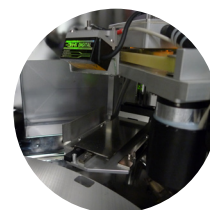
Adjustment of handling system to different labware: • T-flasks • Tip boxes • Petri dishes
