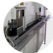
Customize accessories like transfer connection shuttle in-between Cytomat devices
