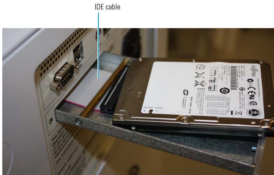
Figure 95. Hard drive unplugged from the IDE cable
