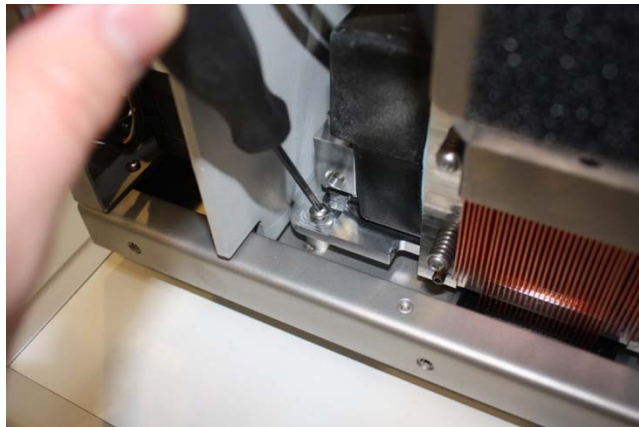
Figure 134. Securing the back left screw
