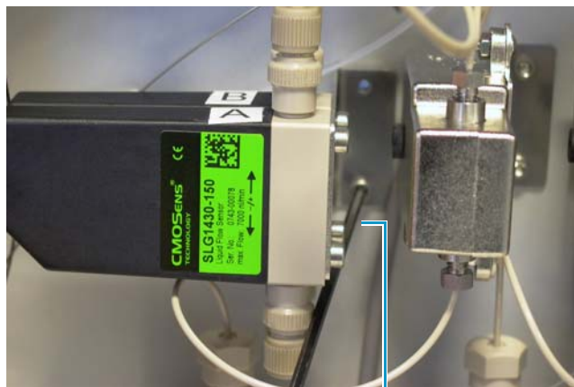
Figure 171. Removing the two screws that secure the flow sensor bracket to the panel
