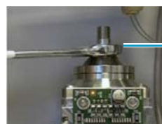
Figure 3. Removing the pump head
