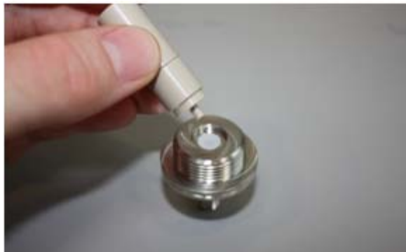
Figure 57. Piston seal properly seated in the pump head (PLF model pump)
