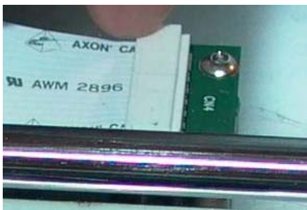
Figure 148. Cap around the ribbon cable (close-up view)
