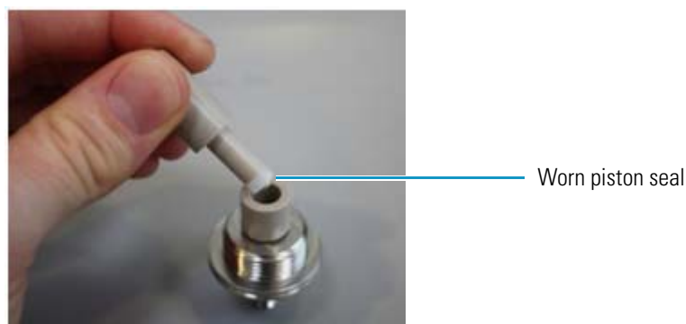
Figure 52. Using the piston seal tool to remove the worn piston seal (PLF model pump)
