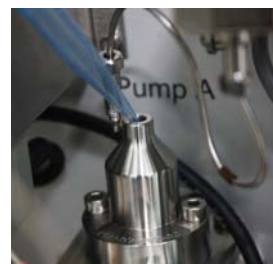
Figure 7. Adding solvent to the pump head
