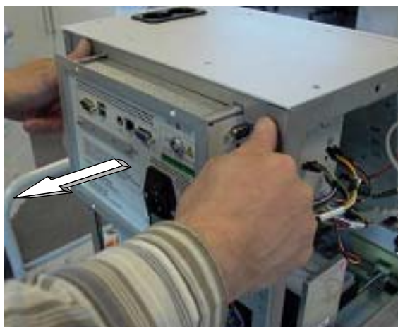
Figure 102. Pulling out the computer box
