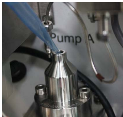
Figure 65. Adding solvent to the pump head
