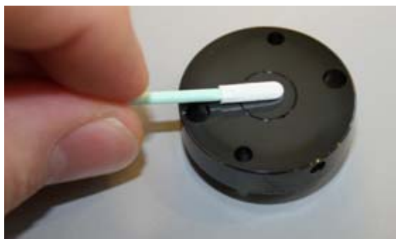
Figure 67. Cleaning the stator
