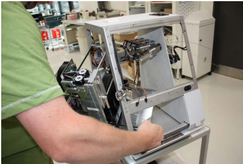
Figure 125. Putting in the ASC autosampler
