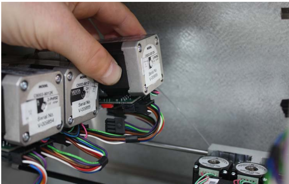
Figure 160. Pulling out a valve
