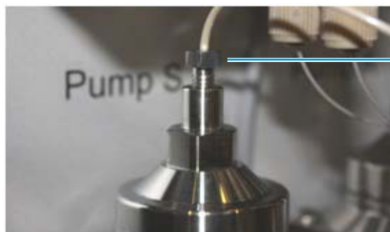
Figure 49. Internally threaded pump head for a PLF model pump
