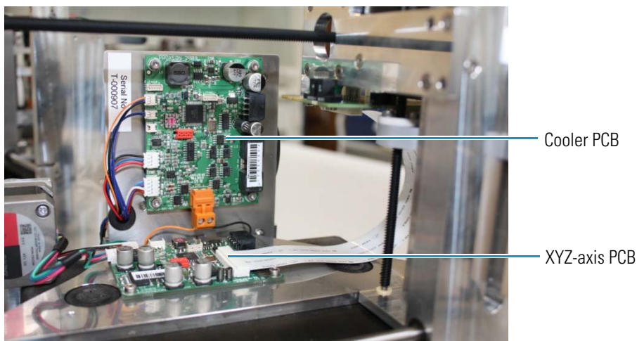
Figure 130. Boards that the P-Bus communication cables connect to
