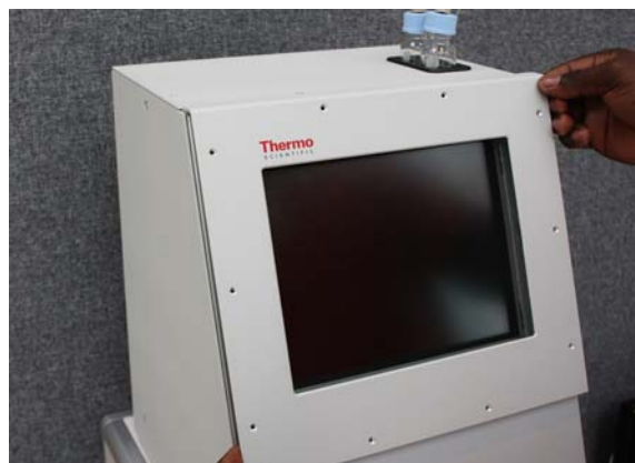
Figure 103. Removing the front plate from the EASY-nLC II instrument
