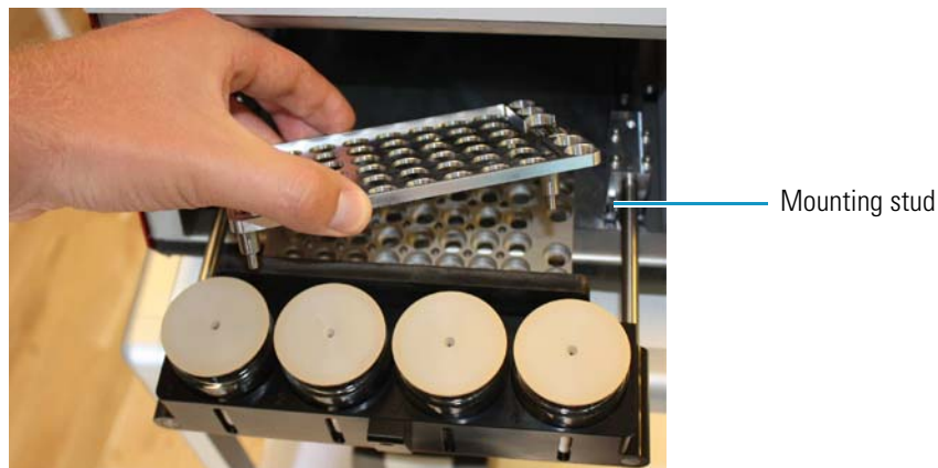
Figure 238. Removing the vial adapter plate before installing the microwell plate adapter plate
