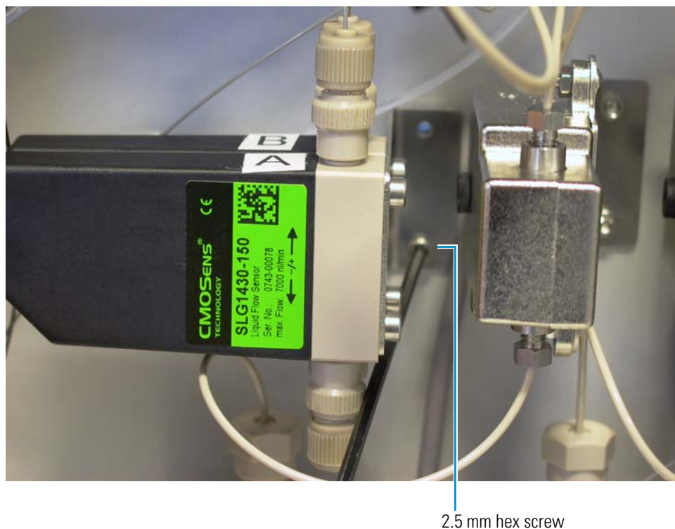
Figure 87. Removing the two screws that secure the flow sensor bracket to the panel
