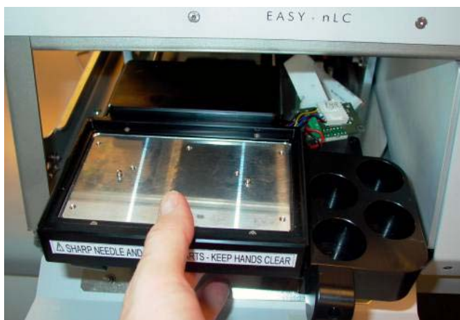
Figure 154. Pulling the adapter plate holder out of the autosampler
