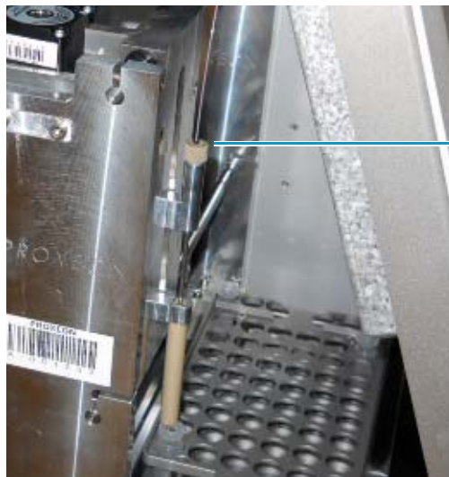
Figure 246. O-ring pushed slightly above the ASC needle holder
