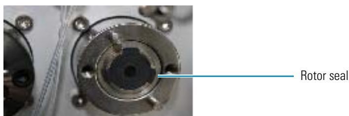
Figure 68. Rotor seal mounted on the valve driver
