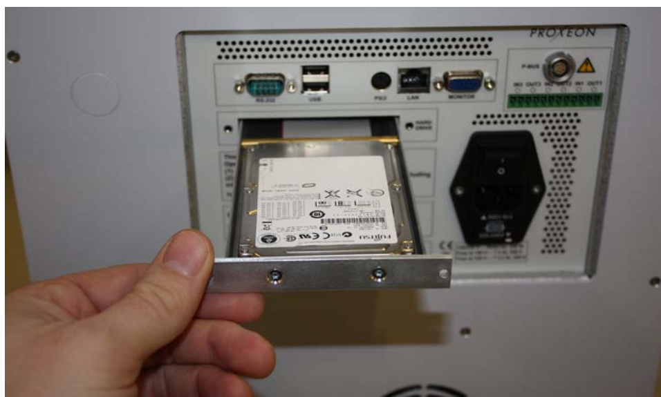
Figure 93. Pulling out the hard-drive drawer
