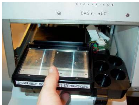
Figure 157. Placing the new cooler in the autosampler bed
