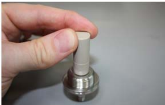
Figure 56. Seating the piston seal (PLF model pump)
