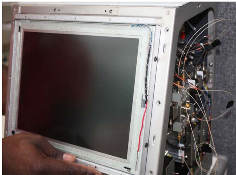
Figure 107. Removing the monitor
