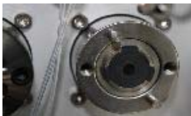
Figure 1. Rotor seal mounted on the valve driver
