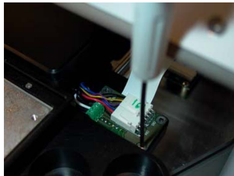
Figure 152. Loosening the screw in the middle left side
