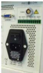
Figure 45. Replacing the main power fuse
