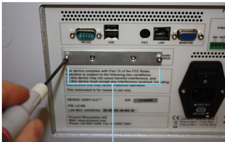
Figure 92. Screws that secure the hard-drive drawer (obsolete computer box shown)
