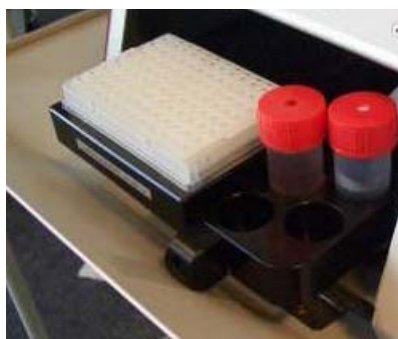
Figure 239. Tray compartment of the ASA model autosampler
