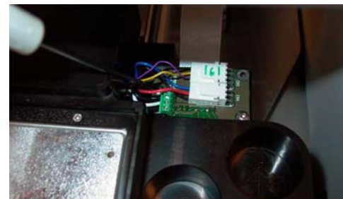
Figure 152. Loosening the screw in the middle left side
