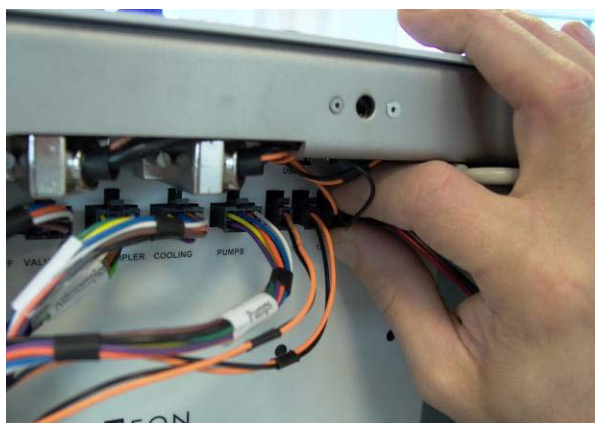
Figure 99. Pressing the tab on the top of the plug of the 12 V cables
