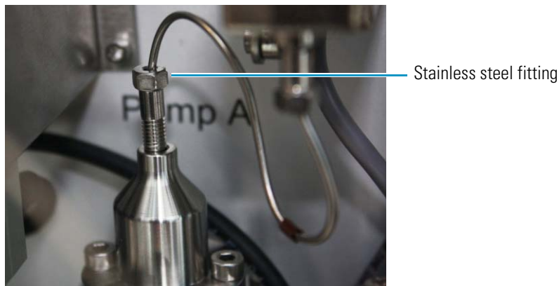
Figure 58. Stainless steel fitting connected to the pump head (PLU model pump)
