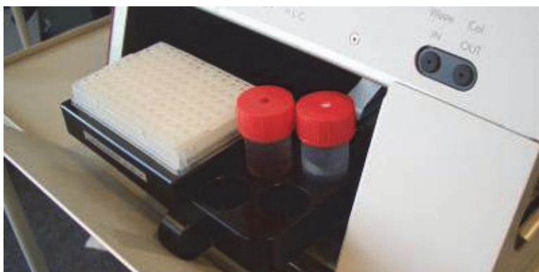
Figure 3. Tray compartment for the earlier version of the EASY-nLC II instrument with an ASA model autosampler (viewed from above)
