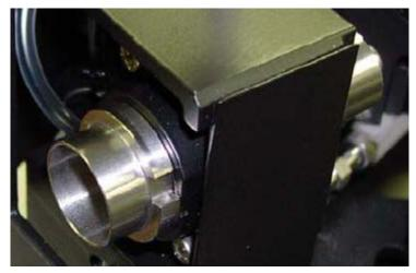
Make sure the cone is started straight in the hole. If the cone enters the electrode mis-aligned the cone can be damaged and made unusable.
