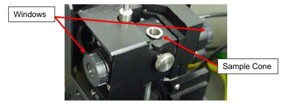
Remove the two windows and the sample cone from the furnace.
