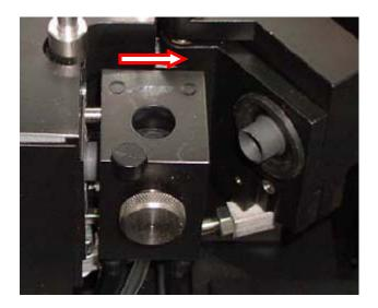
Slide the center block to the left. It is not held in place, but is mounted on two pins. Once the block is off of the pins it can be gently laid down forward. There is no need to disconnect the hoses to the center block.
