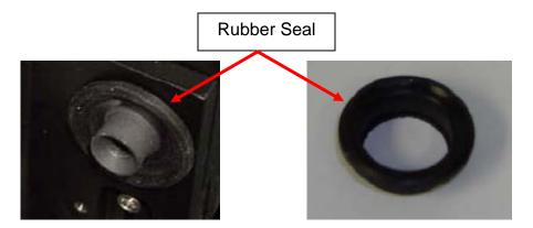
Locate and carefully remove the rubber seal around the right hand cone.
