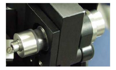
Now repeat the process for the right hand cone. Replace the rubber seal around the right hand cone once the insertion tool has been removed.
