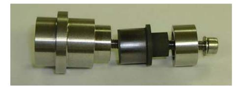
This picture is shown for referencing the orientation that the cone parts of the insertion tool will be assembled.
