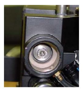
Insert the screw into back of the cone so as shown in the picture above. The screw head should be facing where the window would be.
