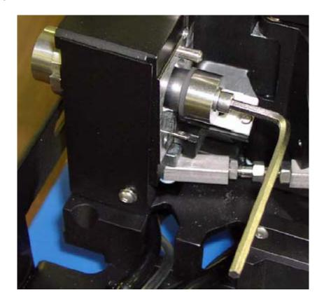
The cone should be inserted until the shoulder ring is snug against the metal surface of the electrode. The screw will show a very large resistance to turning at that point.
