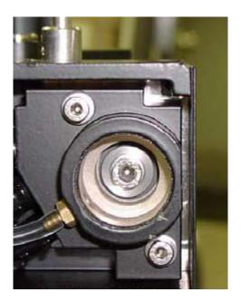
The major difference between the right and the left side removal is the position of the cap is such that the pin will fit into a notch cut into the cap. See the picture below.
