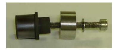
Assemble the screw, washer and insertion cap as shown in the picture above. The flat side of the insertion cap should be towards the head of the screw.
