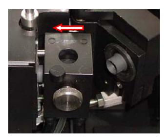
Replace the sample cone in the block. Insert a new cuvette and the furnace is now ready for operation.
