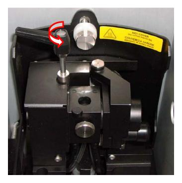
Rotate the handle to open the furnace. If the cuvette is still present in the furnace, remove it from the furnace.
