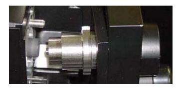
The cap should fit over the cone from the opposite side. Now using the Allen wrench supplied tighten the screw to draw the cone from in the electrode into the cap. Continue until the cone is free of the electrode. Remove the screw from the cap. The cone has now been removed.
