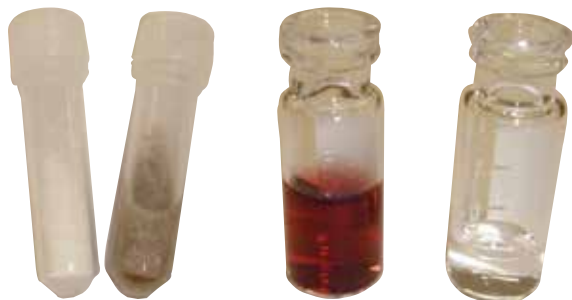
Figure 1: Top: dSPE tubes with 150mg MgSO_4 and 150mg PSA before and after cleanup of 1mL red wine extract; Bottom: Red wine extract before and after dSPE cleanup.
