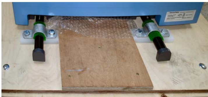
Figure 2-5. Carry handles, fixed on the transport pallet
