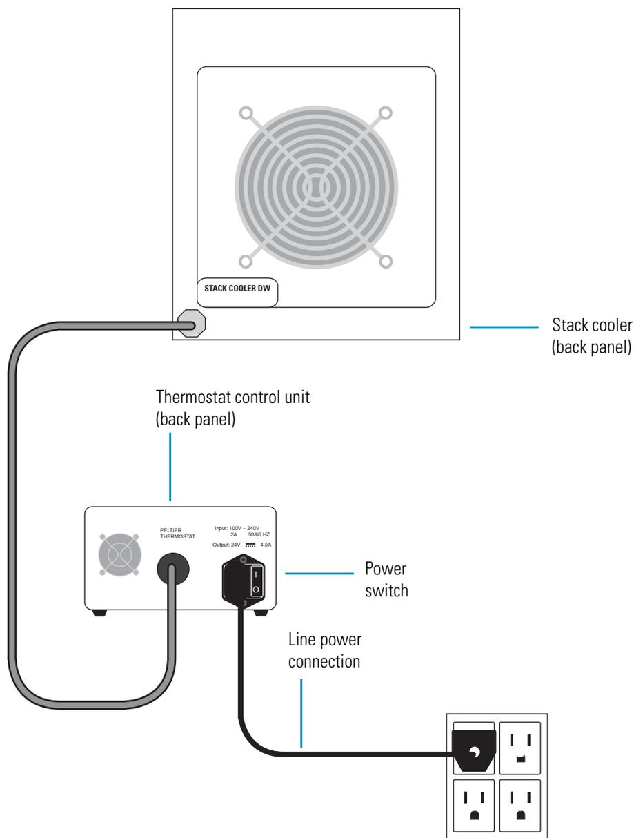
[Figure 30](#) shows the line power connections for an Accela LC system with an Accela Open Autosampler.
