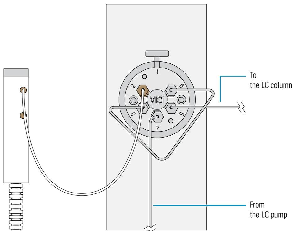
4. Using a 1/4 in. open-end wrench, tighten the fitting.
