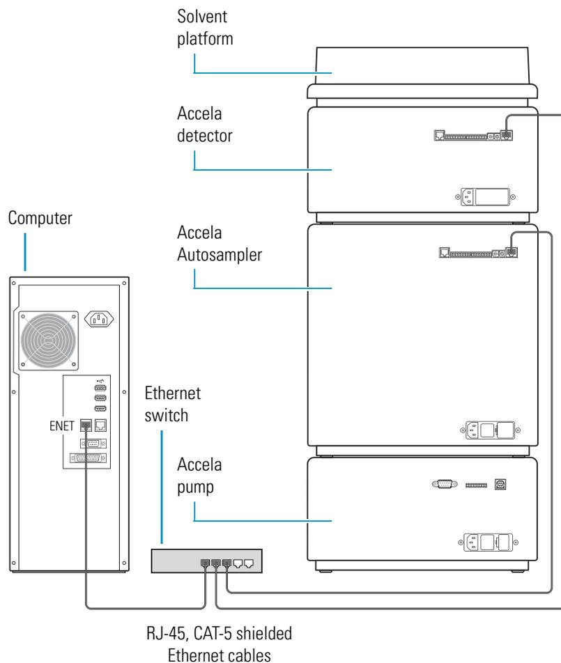
2. To connect the Ethernet switch to the data system computer (see [Figure 22](#)), do the following:
