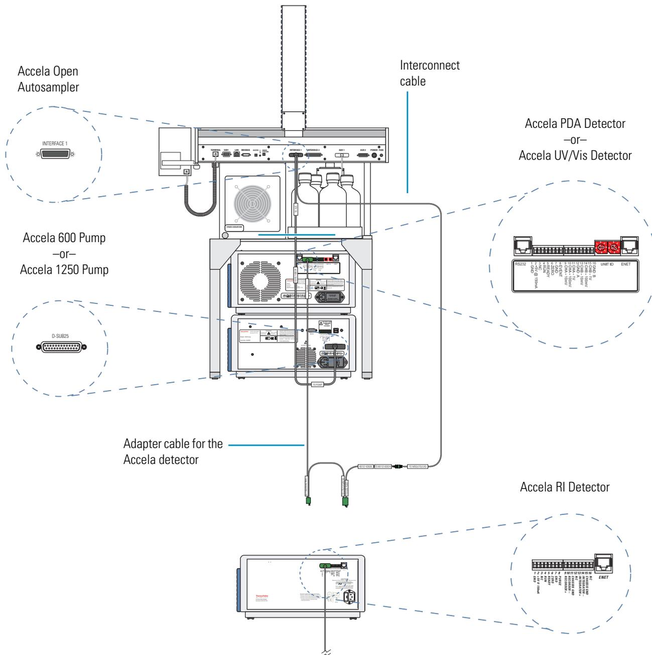
**Figure 18.** Accela Open Autosampler interconnect cable and detector adapter cable connections
