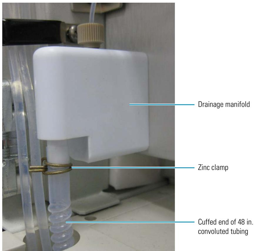
3. Attach the cuffed end of a 0.9 m (36 in.) length of convoluted tubing to the drain port on the bottom of the pump and place the other end of the tubing into an appropriate waste container.
