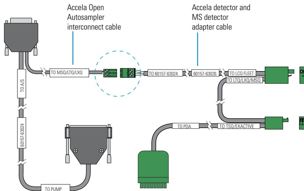
3. Using the adapter cable connectors, make the appropriate connections to an Accela detector, a Thermo Scientific mass spectrometer, or both as follows:
