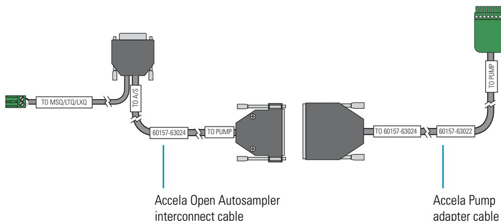
3. Connect the 8-pin connector of the Accela Pump adapter cable to pins 1 through 8 on the back panel of the Accela Pump (see [Figure 21](#)).
