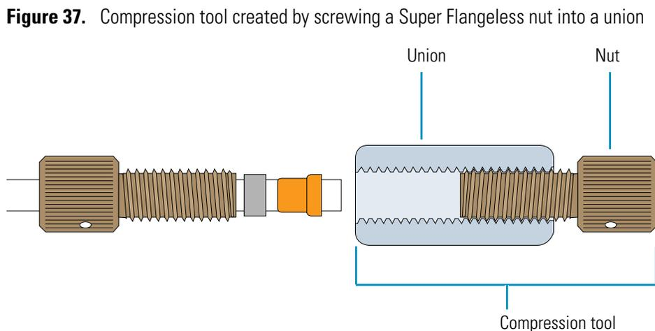
**Figure 37.** Compression tool created by screwing a Super Flangeless nut into a union
