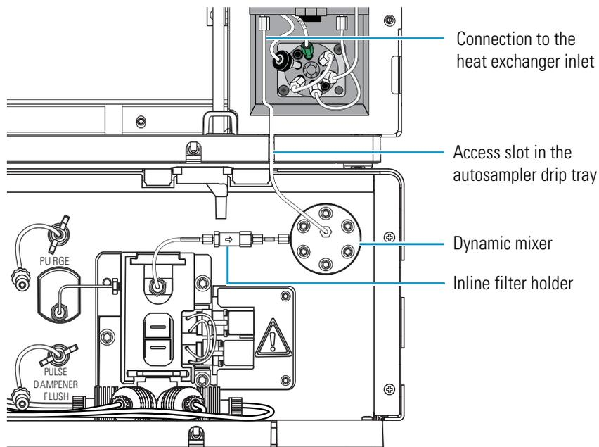
**Figure 46.** Connection between the Accela 600 or Accela 1250 Pump and the Accela Autosampler
