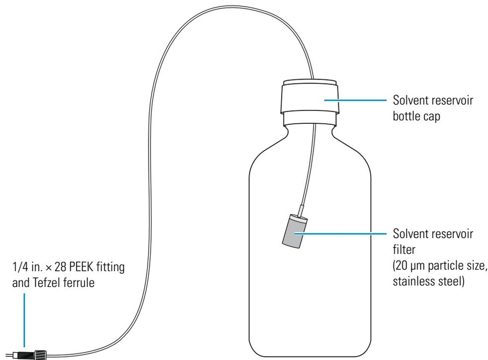
**Note** Each solvent line has a different color fitting. The colors are yellow, green, orange, and blue. Matching the color of the inlet line fitting to the outlet line fitting is important for ensuring that the correct solvent goes into and out of the degasser lines and into the inlet ports of the pump proportioning valve.
