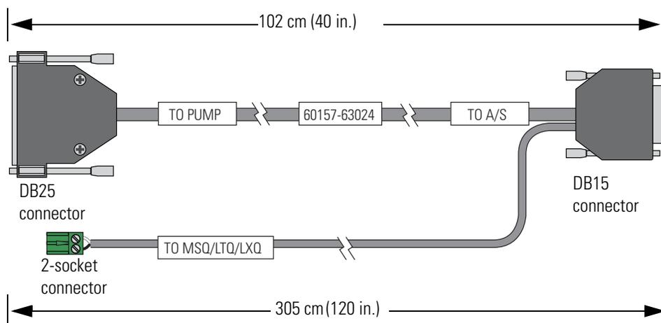
❖ **To connect the Accela Open Autosampler interconnect cable (or equivalent) to the LC or LC/MS system modules**
