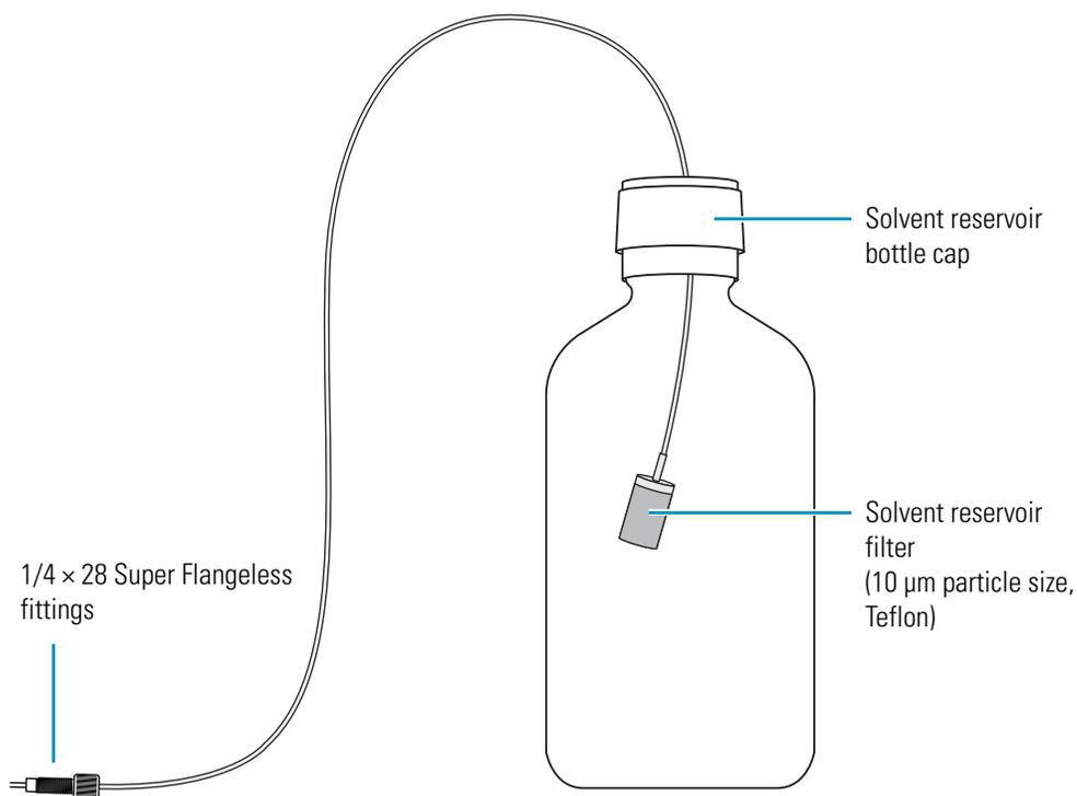
5. Insert the solvent reservoir filter and inlet line into one of the solvent reservoir bottles, and screw the cap onto the solvent reservoir bottle until it is secure.
