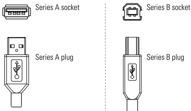
2. Connect the series B plug to the port marked USB on the back of the Accela pump.
