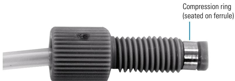
5. Insert the tubing with the properly swaged fitting into inlet port A, and then tighten the nut fingertight. Be careful not to cross-thread the fitting, which can cause solvent leakage (see [Figure 16](#)).
