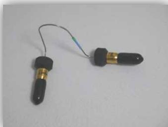
*Fig. 7: Capillary from the pump head to the flow meter inlet*
