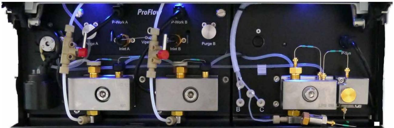
*Fig. 9: Detail view of NCS-3500RS pump module with installed ProFlow flow meter*
