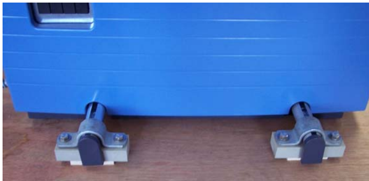
Figure 2-2. Retractable handles for transport, fixed on the transport pallet
