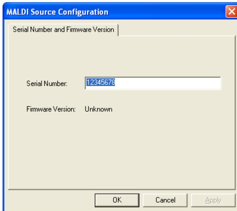
The Serial Number box contains the current entry for the serial number, and the Firmware Version readback displays the firmware version of the MALDI source. The Firmware Version readback displays a value of Unknown until you run the Tune Plus MALDI diagnostics tool for the first time.
