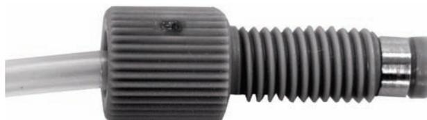
3. Insert the tubing with the properly swaged fitting into inlet port A, and then tighten the nut finger-tight. Be careful not to cross-thread the fitting, which can cause solvent leakage.
