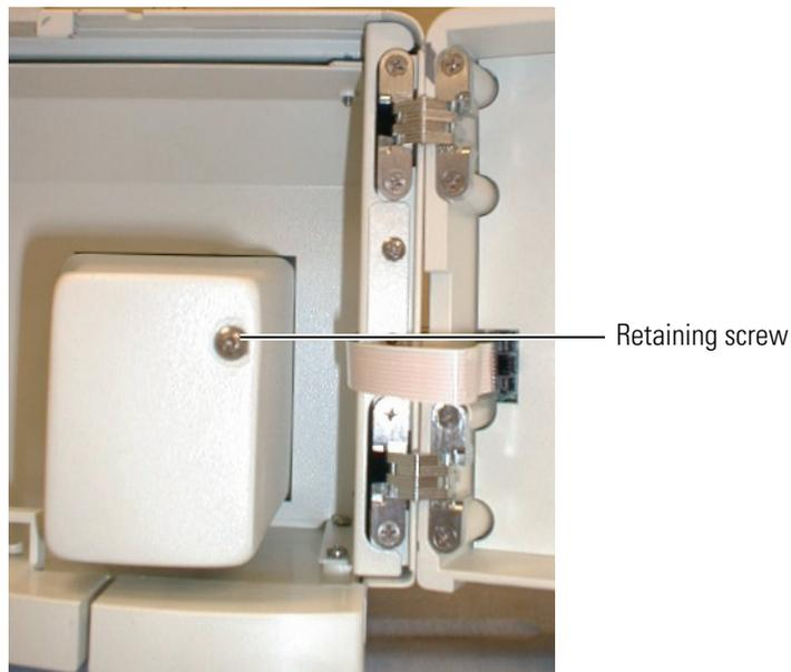
3. Remove the sample photodiode from the end of the mounting assembly. Use an Allen wrench to remove the two screws that secure the sample photodiode to the end of the mounting assembly. See [Figure 63](#).
