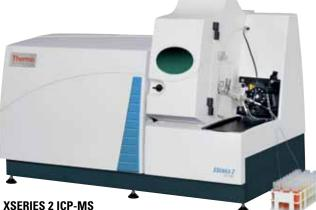
The Thermo Scientific\* XSERIES 2 ICP-MS offers outstanding productivity in a quadrupole ICP-MS for both routine and high performance analytical work.
