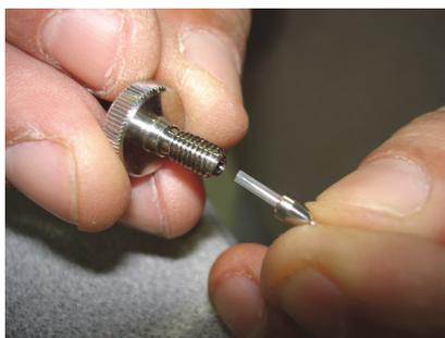
3. Install a new needle seat into the needle guide with the metal ferrule pointing away from the needle guide ([Figure 52](#)).
