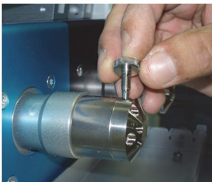
2. Remove the needle seal from inside the needle guide ([Figure 52](#)).
