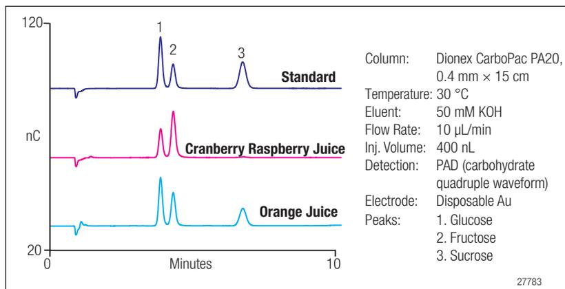
Figure 14. Separation of glucose, fructose, and sucrose in juice samples using a capillary RFIC system.
