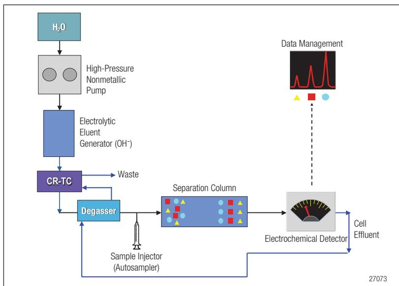
Figure 3. Block diagram of a capillary RFIC system with electrochemical detection.
