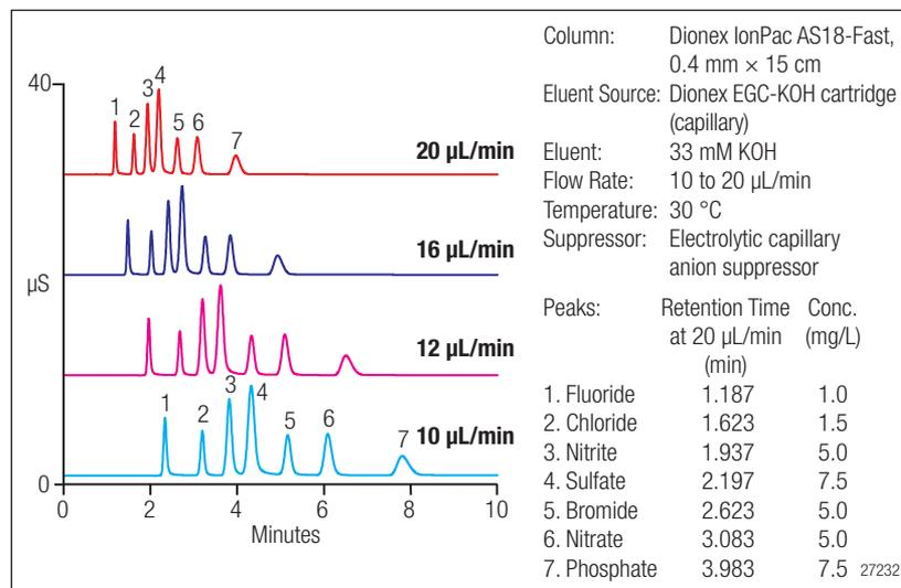
Figure 8. Fast separation of seven common anions on a capillary Dionex IonPac AS18 column.
