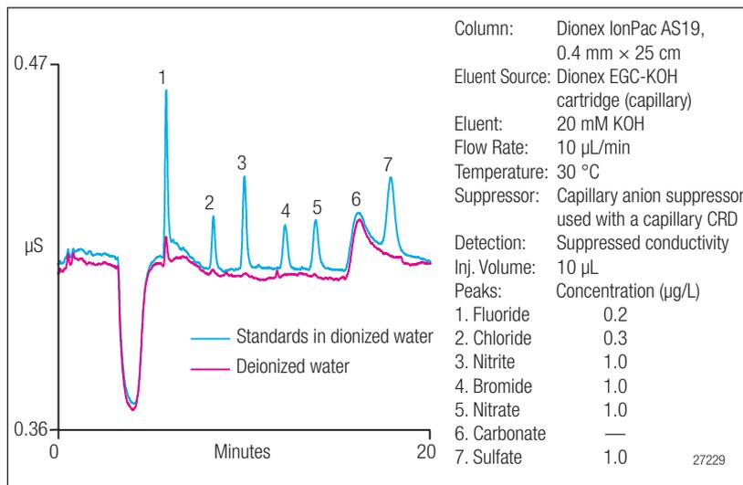
Figure 10. Separation of inorganic anions at trace concentrations on a capillary Dionex IonPac AS19 column with 10  $\mu\text{L}$  injection.
