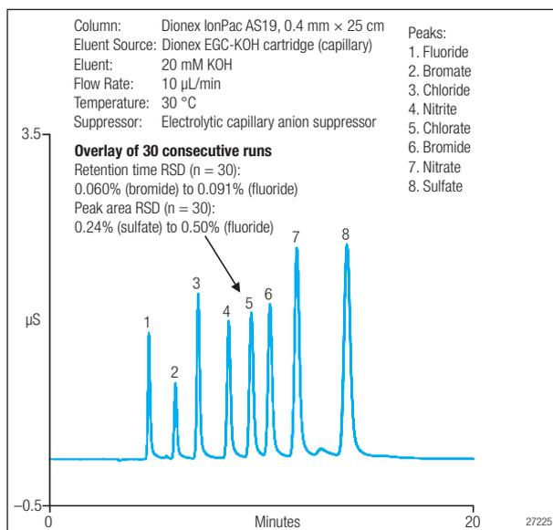
Figure 4. Isocratic separation of common anions obtained using a capillary Dionex IonPac AS19 column.
