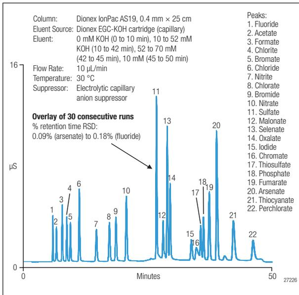
Figure 5. Gradient separation of 22 anions on a capillary Dionex IonPac AS19 column.
