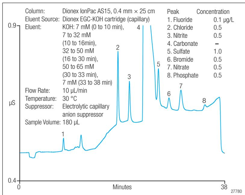
Figure 11. Separation of inorganic anions at trace concentrations on a capillary Dionex IonPac AS15 column with 180  $\mu\text{L}$  injection.
