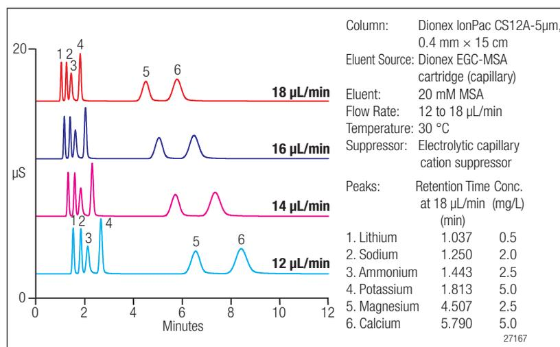
Figure 9. Fast separation of six common cations on a capillary Dionex IonPac CS12A column.
