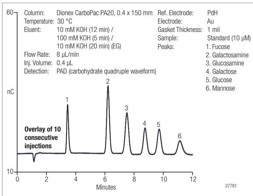
Figure 12. Separation of six monosaccharides.
