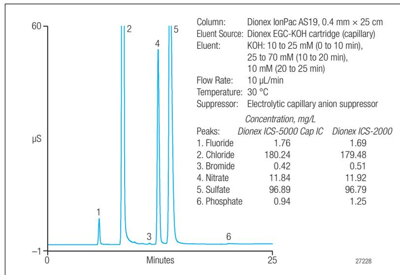
Figure 7. Determination of common anions in a treated wastewater sample.
