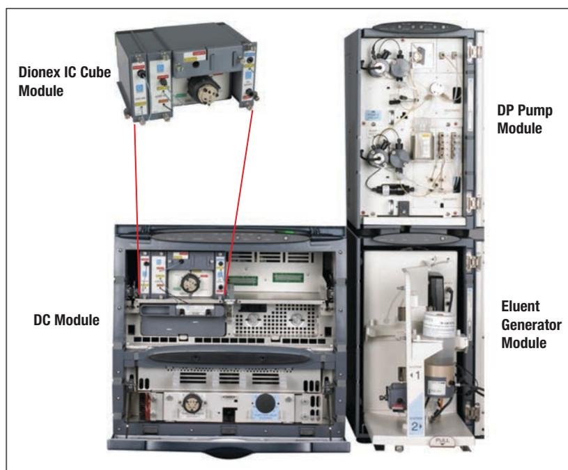
Figure 1. An ICS-5000 capillary RFIC system.
