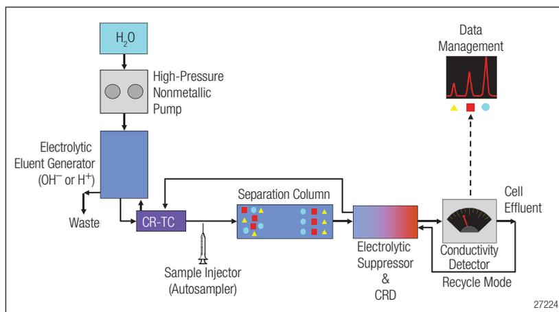
Figure 2. Block diagram of a capillary RFIC system with suppressed conductivity detection.
