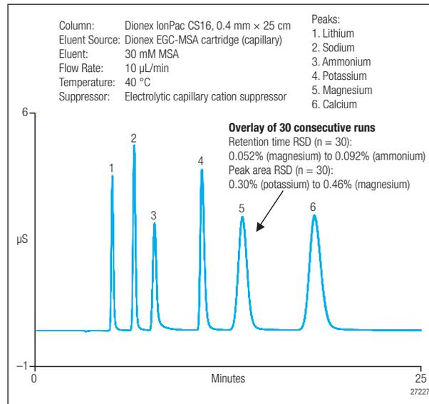
Figure 6. Separation of common cations obtained using a capillary Dionex IonPac CS16 column.
