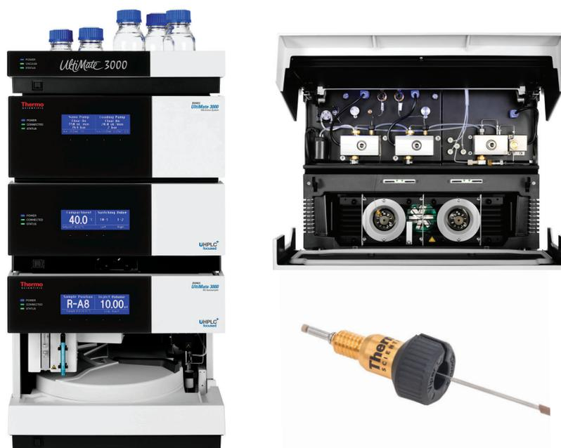
Figure 3. UltiMate 3000 RSLCnano system, interior view, and nanoViper fitting.
