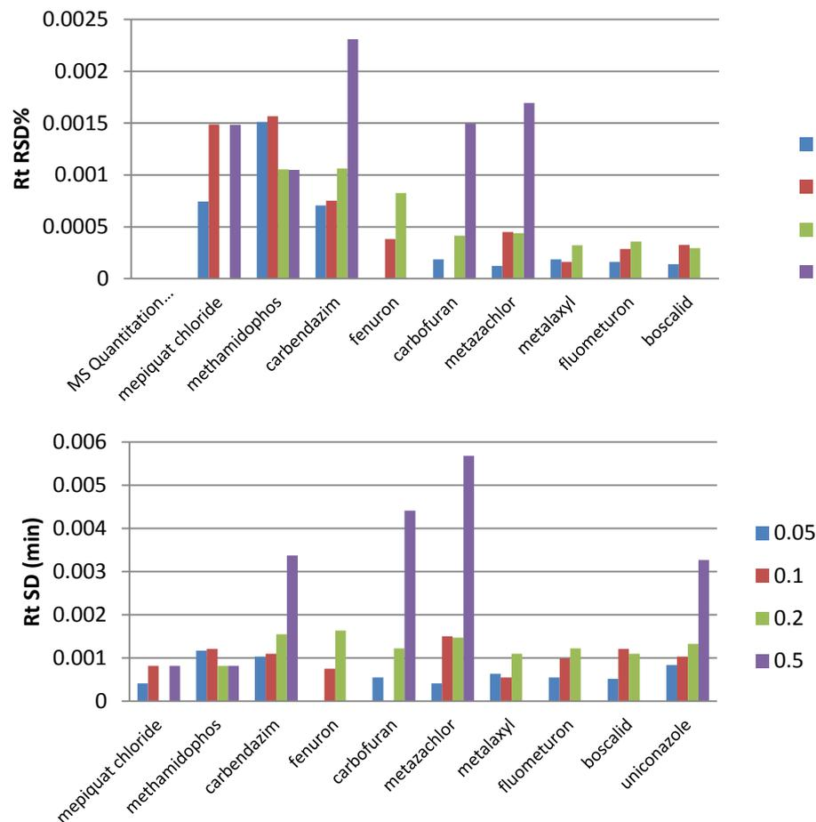
Data rates of at least 10 Hz are necessary to achieve a retention time precision of SD=0.001 min (RSD% < 0.1%) for peaks with a half-height width of 0.025 min (1.5 s).
