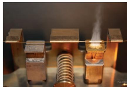
Figure 2: CO<sub>2</sub> Modulator (located inside the GC oven) resulting in loss of information or the focussing of chromatographic noise along with the peak of interest.
