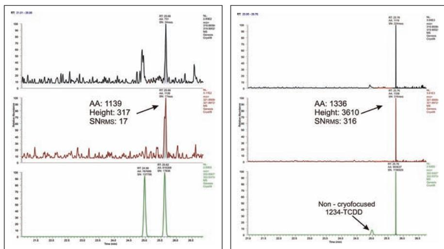
Figure 7: sensitivity increase with CZC in 1/10 EPA 1613 CSL standard (10 fg/μL 2378-TCDD); left - standard chromatogram TCDD (mass trace 1 and 2: ratio/qualifier and quantification m/z for native (<sup>12</sup>C) TCDD; trace 3: quantification m/z <sup>13</sup>C TCDD); right - chromatogram with cryo-focussed 2378-TCDD peaks, note: 1234-TCDD is not focussed.
