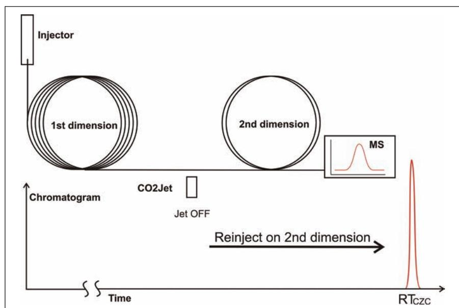
Figure 5c: Cryogenic jet off: step 2 – re-inject peak of interest on 2<sup>nd</sup> dimension column
