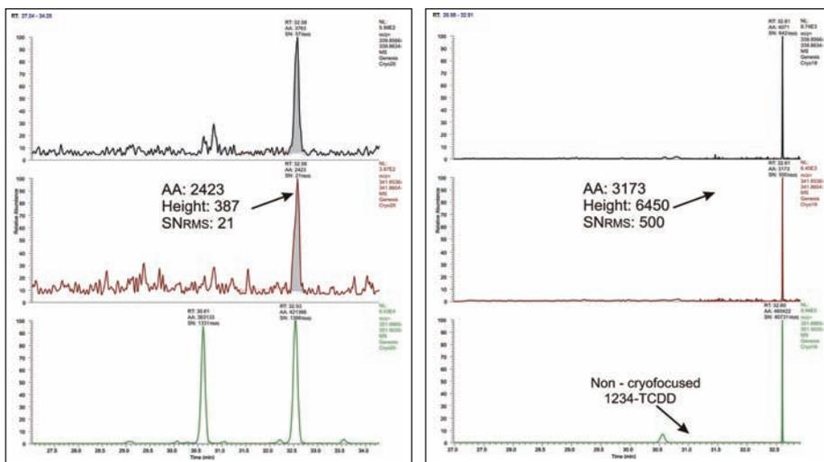
Figure 9: sensitivity increase for native PCDF with CZC in low level pooled blood sample ca. 30 fg PCDF; left - standard analysis; right - CZC experiment; mass traces analogue to Figure 7, only for PCDF
