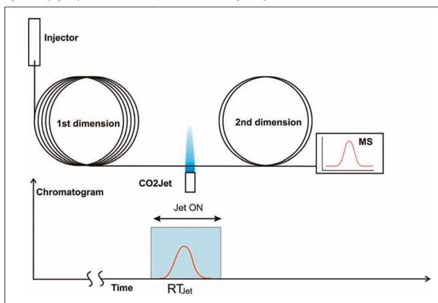
Figure 5b: Cryogenic jet on: step 1 – cryo-traps whole 1<sup>st</sup> dimension peak of interest
