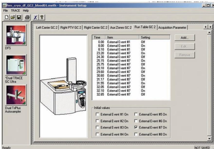
Figure 3: GC time events to control cryogenic jet
