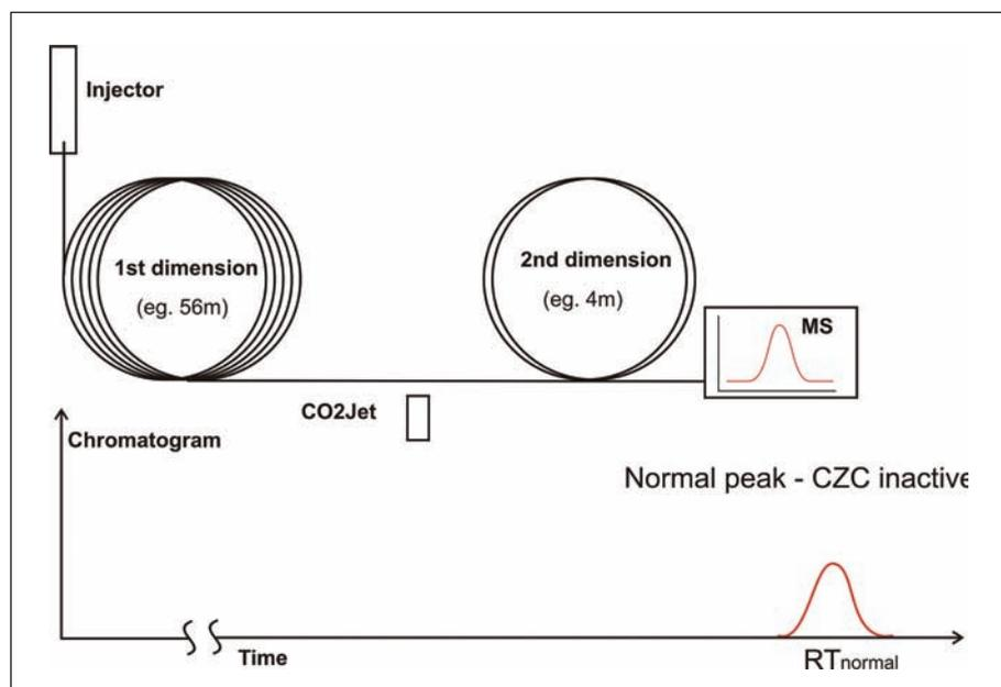
Figure 5a: Cryogenic jet off results in normal peak width for non-target analytes
