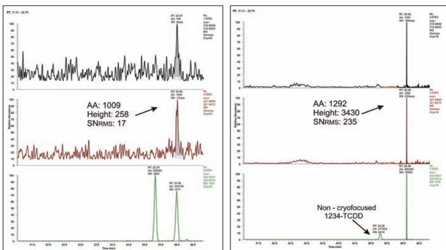
Figure 8: sensitivity increase for 2378-TCDD with CZC in low level pooled blood sample (ca. 10 fg/μL native TCDD); left - standard analysis; right - CZC experiment; all mass traces as explained in Figure 7
