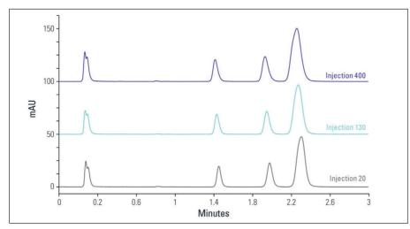
Figure 14: Accucore column stability at 70° C. Experimental Conditions: Column - Accucore C18 2.6µm, 100 x 2.1mm; Mobile phase: 35:65 (v/v) Water/Methanol; Flow rate: 400µL/min; Injection volume: 1.5µL; Temperature: 70°C; Detection: UV at 254nm (0.1s rise time, 20Hz); Order of elution: 1. Theophylline/Caffeine (t0), 2. Phenol, 3. Butylbenzene, 4. o-Terphenyl, 5. Pentylbenzene/Triphenylene.
