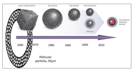
Figure 1: Particle evolution: packing materials have changed from large pellicular particles via smaller totally porous particles to spherical particles with diameters of less than  $2\mu$ m, to 2.6 $\mu$ m solid-core particles
