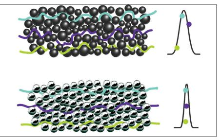
Figure 2: Representation of the effect of average particle size distribution (D90/10) on the packed bed homogeneity and band broadening through Eddy diffusion. Top - D90/10 ~ 1.5; Bottom - D90/10 ~ 1.1.
