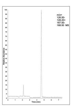
Figure 10. Separation of melamine and cyanuric acid on Accucore HILIC. Experimental conditions: Column Accucore HILIC 2.6µm, 150mm x 4.6mm; Mobile phase: 90:10 (v/v) Acetonitrile:50mM Ammonium Acetate, pH 5; Flow rate: 1mL/min; Temperature: 40°C; Detection: MS at m/z 127, 128, 168 (negative mode 0-3 mins, positive mode 3-10 mins); Injection volume: 5µL; Backpressure: 117 bar; Analytes: Cyanuric Acid: m/z 128.1 (-1) Melamine: m/z 127.1 (+1), 168.1 (+1 with Acetonitrile adduct).
