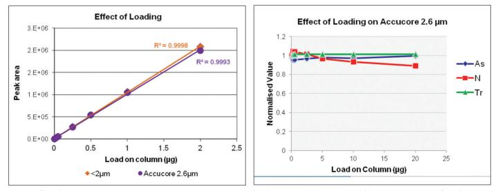
Figure 6: Effect of column loading on chromatographic parameters. (a) Comparison of loading 2µg on solid-core 2.6µm and fully porous sub-2µm; (b) Effect of loading on peak asymmetry (As), retention time (Tr) and efficiency (N) on the solid-core column.
