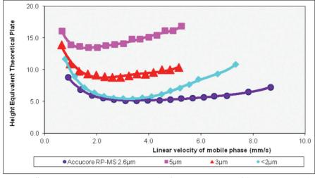
Figure 3: Efficiency comparison using Van Deemter plots for Accucore 2.6µm and fully porous 5, 3 and sub-2µm.
