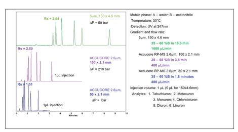
Figure 7. Example of method transfer from fully porous 5µm 150x4.6mm column to Accucore 2.6µm, 100x2.1 ID mm column (similar column chemistry)
