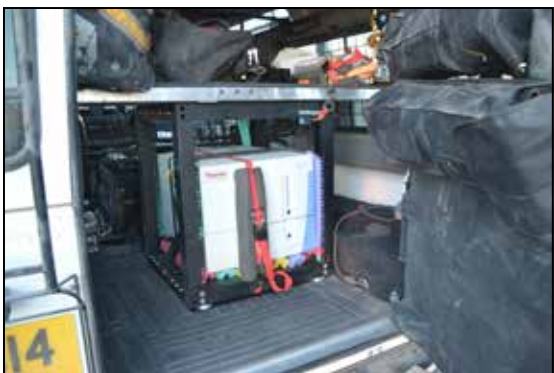
Figure 3a: Photograph of the Delta Ray IRIS installed at the back of our field vehicle.
