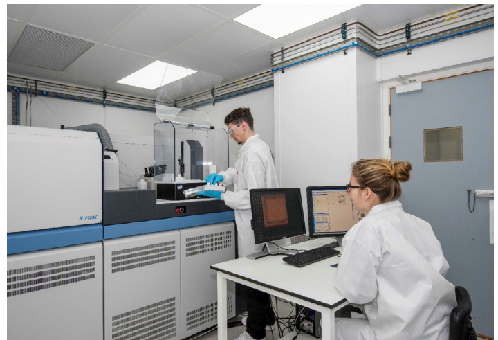
Figure 3. Elwyn de la Vega (standing) running boron isotopes on foraminifera on the Neptune MC-ICP-MS 1 in the Geochemistry Laboratory of the School of Ocean and Earth Science, University of Southampton.
