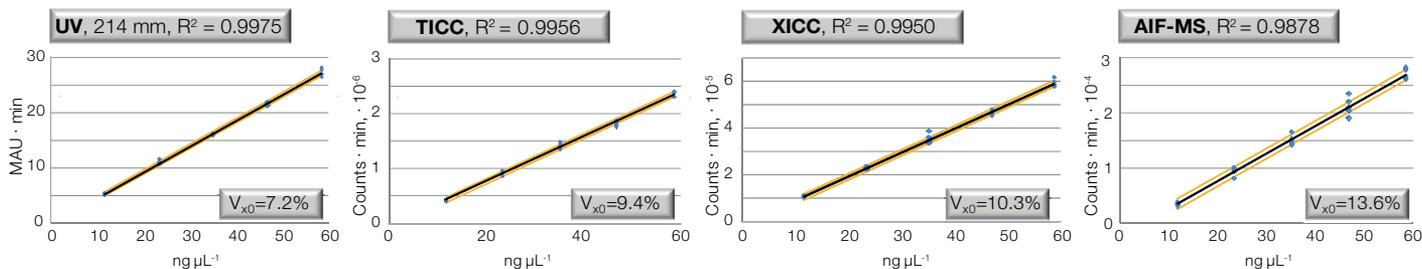
**Figure 4. Calibration curves for the non-oxidized Fc/2 fragment of MabThera (Rituximab) using UV-spectroscopic and mass spectrometric detection.**  $R^2$  = correlation coefficient,  $V_{x0}$  = relative process standard deviation.
