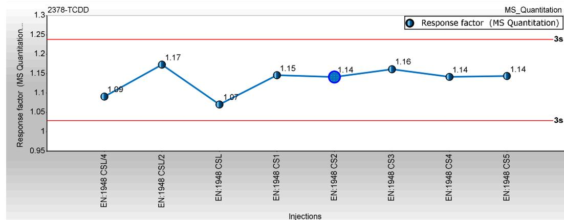
**Example of response factors over 8 calibration injections for 2,3,7,8-TCDD**
