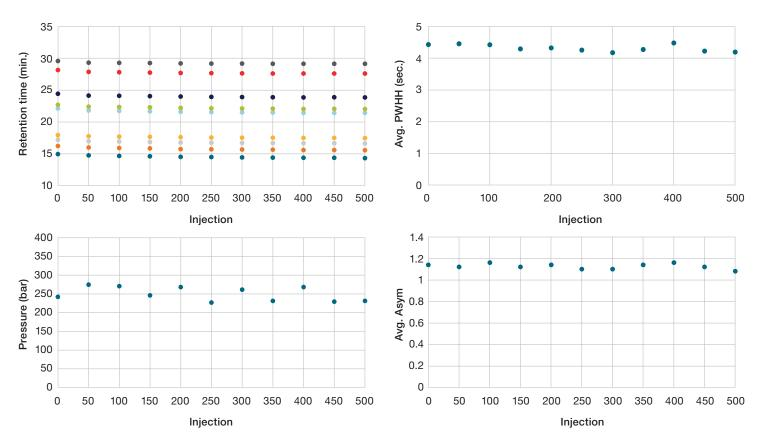
PepMap Neo columns (ES75500PN, 75 μm I.D. x 500 mm) offer excellent robustness: Column ruggedness test from 500 injections with the direct injection workflow using 200 ng HeLa digest. The data shows consistent peak retention time, peak width, peak symmetry, and system pressure.
