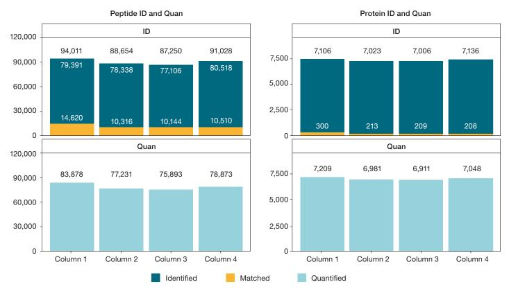
Reproducible identification and quantification using PepMap Neo columns: HeLa peptides and proteins over four EASY-Spray PepMap Neo columns (ES75750PN, 75 µm I.D. × 750 mm) while using the Vanquish Neo UHPLC system (direct injection workflow) coupled with the Thermo Scientific™ Oribtrap™ Exploris 480 Mass Spectrometer. The reproducibility of these columns has been reported in Thermo Scientific Technical Note (TN74152).
