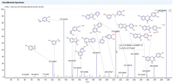
Figure 4. Highly curated data are noise filtered, recalibrated and include annotation of structure, formula, and neutral loss. Manual data curation ensures high quality of all library contents, enabling scientists to achieve greater confidence when identifying unknowns.
