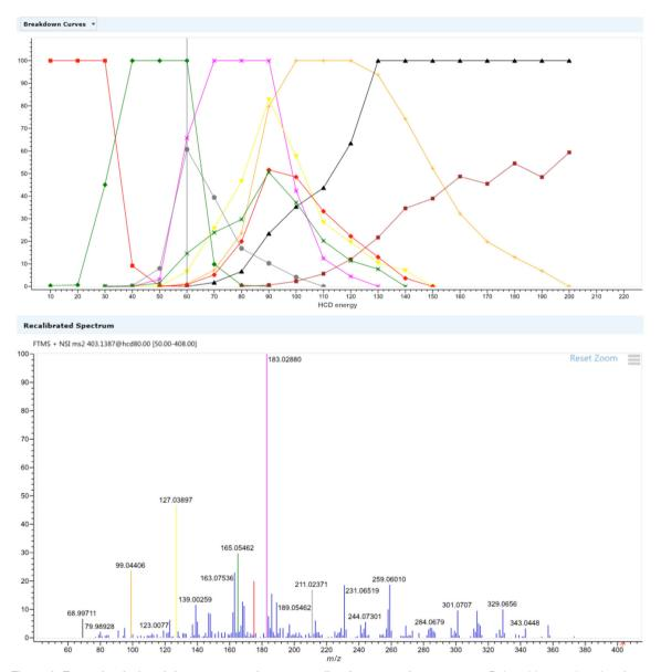
Figure 3. Example of a breakdown curve and corresponding fragmentation spectrum. Being able to review data from multiple fragmentation types and collision energies for each compound facilitates rapid method development for optimal fragmentation acquisition energies.
