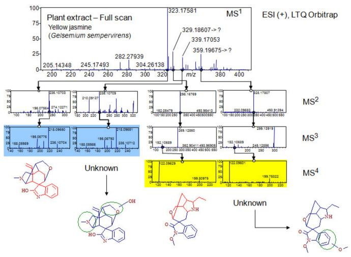
**Figure 7.** An example of how structural similarity, or sub-structure searching can aid in compound identification. Even when an unknown yields no search results, comparing experimental fragmentation spectra to the extensive fragmentation information in mzCloud can yield sub-structural matches that aid in putative identification, with mzLogic using this information to rank proposals, aiding the identification process.
