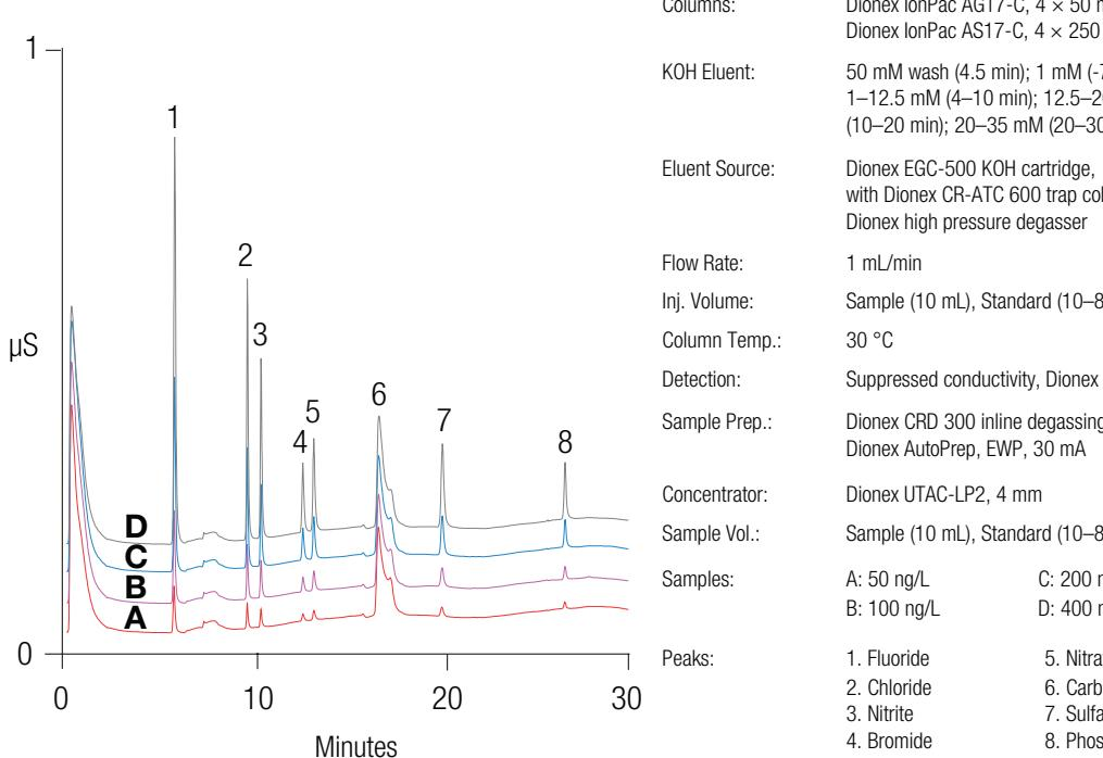
Figure 3. Calibration standards of 50 to 400 ppt on a system utilizing the Thermo Scientific™ Dionex™ AERS™ 500 Anion Electrolytically Regenerated Suppressor in recycled water mode.
