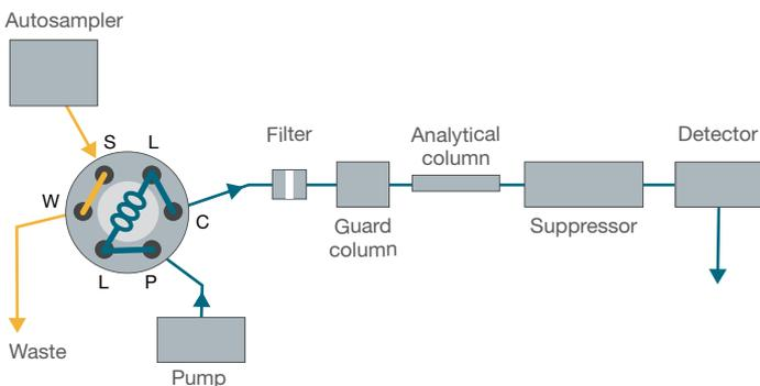
Figure 3. Inline high-pressure filtration schematic.
