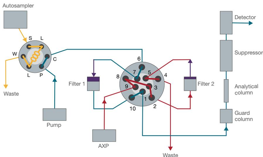
Figure 4. Inline high-pressure filtration schematic, dual filter with backflush.
