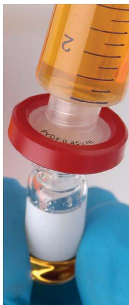
However, being single-use only, syringe filters can be costly and can contribute to a lot of waste. Additionally, there is a potential for them to burst when subjected to high pressure, as can be applied by technicians who are trying to filter high particulate samples.
