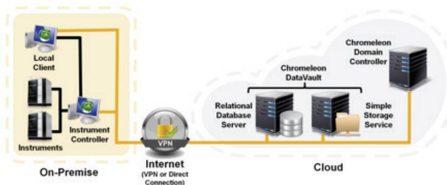
Figure 3. Chromeleon CDS Cloud Deployment Example
