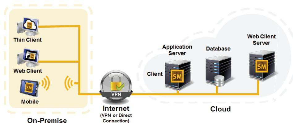
Figure 5. SampleManager LIMS Cloud Deployment Example
