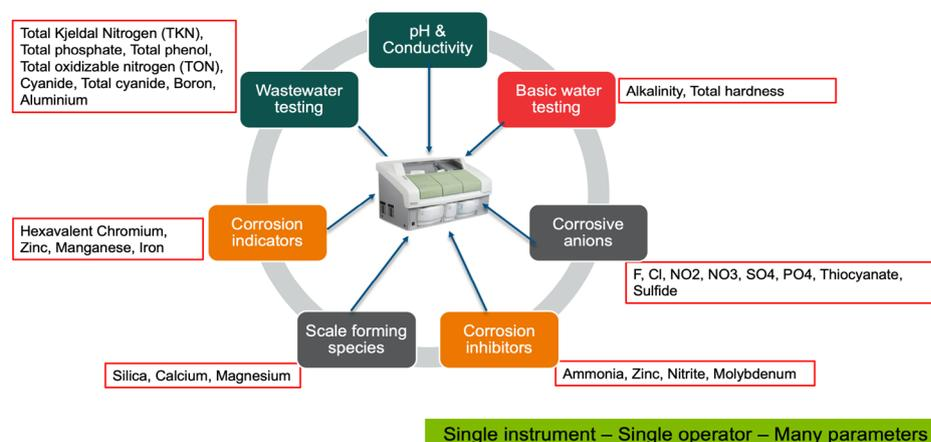
Figure 10: Example analyses performed by the Thermo Scientific™ Gallery™ Plus Discrete Analyzer.
