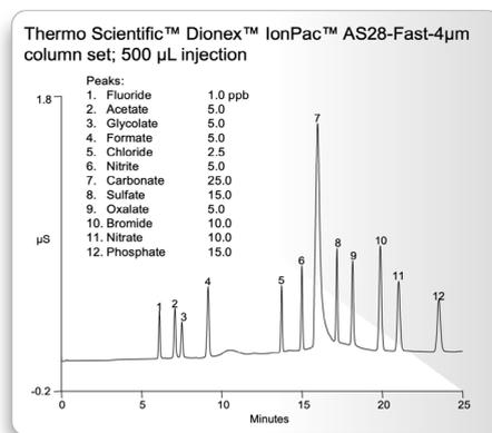
**Figure 6:** Achieving ppt-level determinations using Thermo Scientific™ Dionex™ IonPac™ AS28-Fast-4μm column set (500 μL injection)
