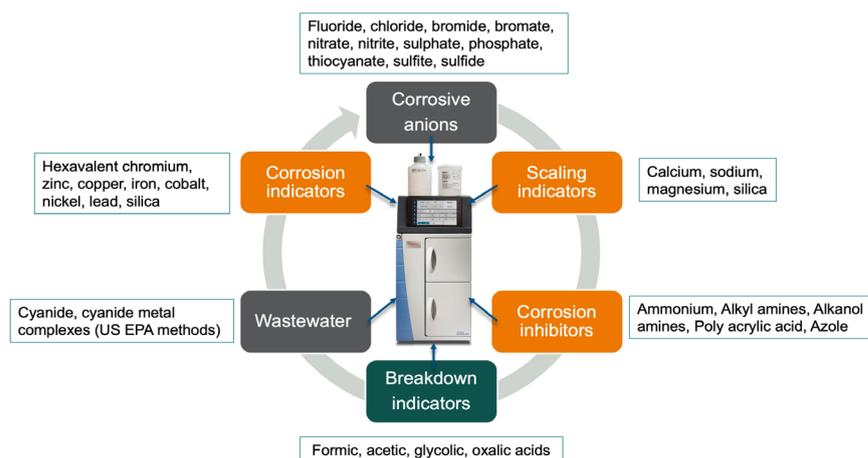
Figure 11: Example analyses performed by Thermo Scientific™ Dionex™ ion chromatography systems.
