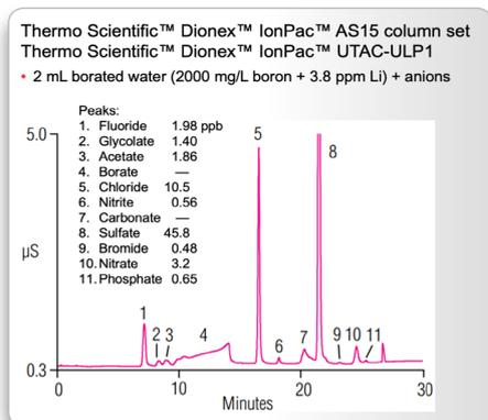
**Figure 9:** Chromatogram of trace ions in water containing higher concentrations of boron and lithium.
