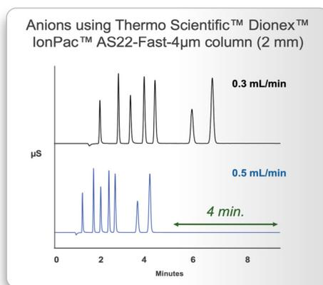
**Figure 4:** Impact of increasing flow rate through the Thermo Scientific™ Dionex™ IonPac™ AS22-Fast-4μm column (2 mm) on the chromatogram of inorganic anions.
