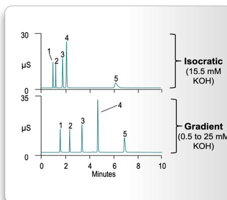
**Figure 5:** Chromatogram of water sample using isocratic versus gradient eluent concentrations.
