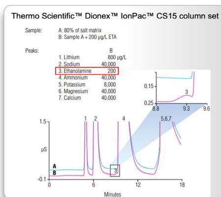
**Figure 7:** Detecting small concentrations of corrosion inhibitors in the presence of larger signals.
