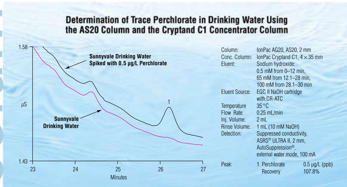
The IonPac Cryptand C1 Concentrator Column is designed primarily for the analysis of trace perchlorate in drinking water. A method using the Cryptand C1 Concentrator Column can quantify 140 ng/L (ppt) of perchlorate in a background of total dissolved solids (chloride, carbonate, and sulfate) at combined concentrations as high as 3000 mg/L. The Cryptand C1 Concentrator Column is the specified concentrator column for sample preconcentration in U.S. EPA Method 314.1.
